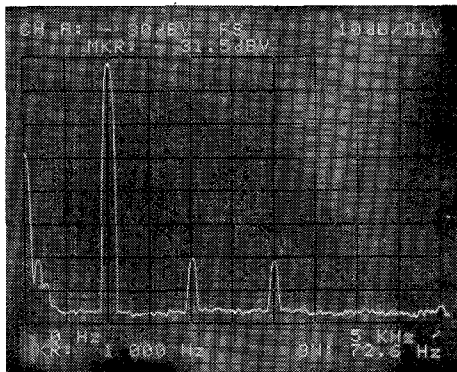
Fig. 11. Spectral contents of a sine wave at the output of the multiplier of Fig. 4.
