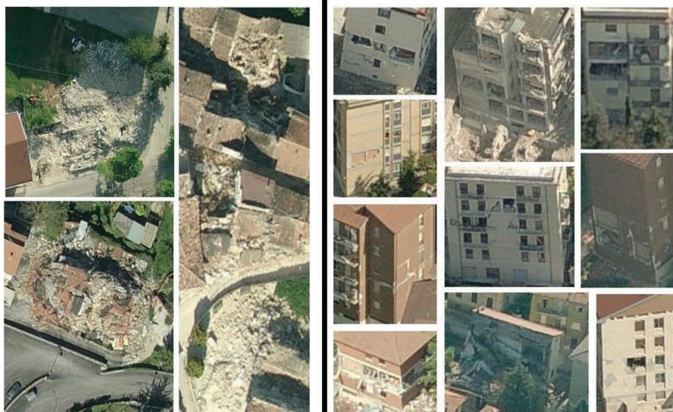
**Figure 1.** Examples of nadir images depicting rubble piles and debris, left. Damaged façades shown in oblique imagery, right.
