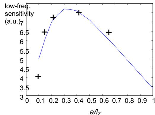
Fig.2 Low-frequency sensitivity  $S(f=0)$  as a function of the ratio  $a/l_z$  (line represents the calculations). The crosses show experimentally obtained results, from devices with  $l_z=240 \mu\text{m}$ ;  $2a=50, 80, 100, 200, 300 \mu\text{m}$ .
