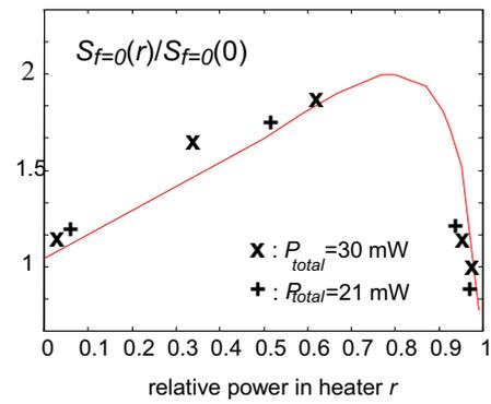
**Fig.5 .** Low-frequency sensitivity  $S_{f=0}$  as a function of relative heater power  $r = P_H / (P_H + 2P_S)$  normalized to the sensitivity  $S_{f=0}$  at  $r=0$ , according to the model calculations (line), and the experimentally obtained points (crosses).
