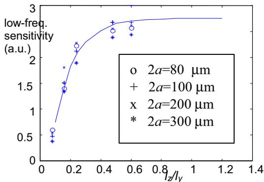
**Fig.3.**  $S(f=0)$  as a function of the ratio  $l_z/l_y$  (line:model). The marks indicate experimentally obtained results from devices with  $l_y = 500 \mu\text{m}$ ;  $l_z = 40, 80, 120, 240$  or  $300 \mu\text{m}$  and  $2a = 80, 100, 200$  or  $300 \mu\text{m}$ .
