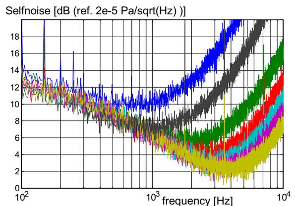
**Fig.6.** Selfnoise levels of the best up to date three-wire type Microflown,  $a = 100 \mu\text{m}$ ,  $l_z = 200 \mu\text{m}$ , a sensor power  $P_{S2} + P_{S1} = 11 \text{ mW}$  and a heater power  $P_H = 0 \text{ mW}$  (upper curve), 5, 10, 20, 32, 44 and 58 mW (lowest curve). The upper curve corresponds to the two-wire configuration.
