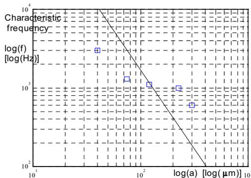
**Fig.4.** Characteristic frequency  $f_c$  of the sensitivity curve, as a function of the distance between the sensing wires, mutual wire distance  $= 2a$ , plotted logarithmically. The line shows the theoretical dependence  $f_c \propto a^{-2}$ .
