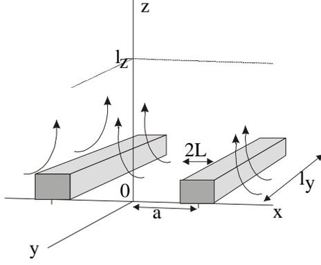
Figure 4. Dimensions of the model of the sensor
