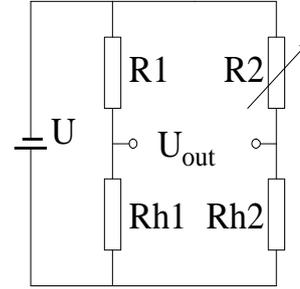
Figure 5 Electronic circuit with  $R1=390\Omega$ ,  $R2=0-1k\Omega$  and  $Rh1 \gg Rh2 \gg 350\Omega$ . and  $U=3V$ .
