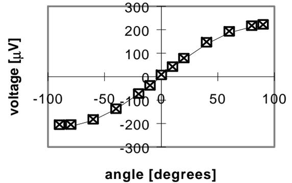
Figure 6 Output voltage versus angle relative to the horizontal.
