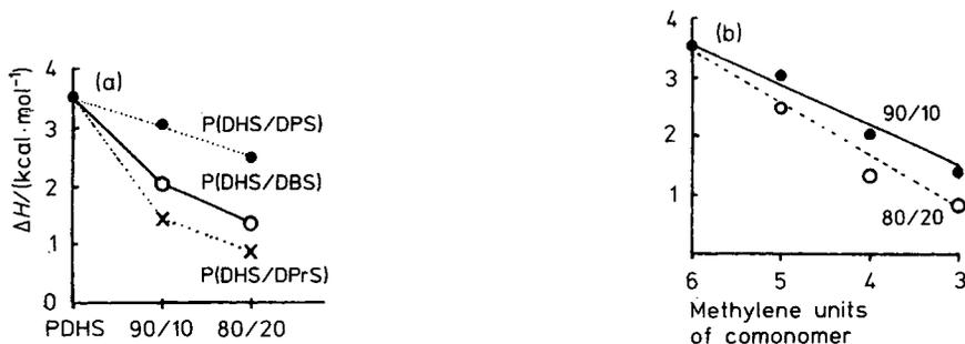
Fig. 5. Transition enthalpies of the copolymers vs. composition **a** and length of side chain of comonomer **b**
