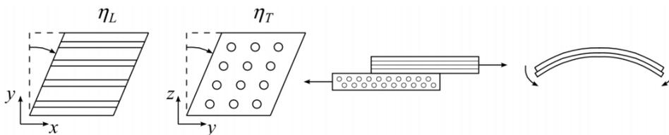
Figure 1: Deformation modes related to the formability of thermoplastic composites. From left to right: intra-ply longitudinal shear; intra-ply transverse shear, inter-ply slip, out-of-plane bending
