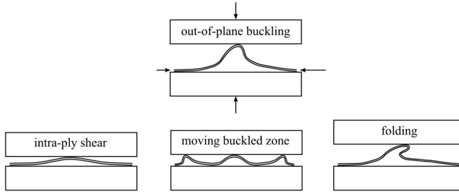
Figure 2: Phenomena originating from out-of-plane buckling upon closing of the tools
