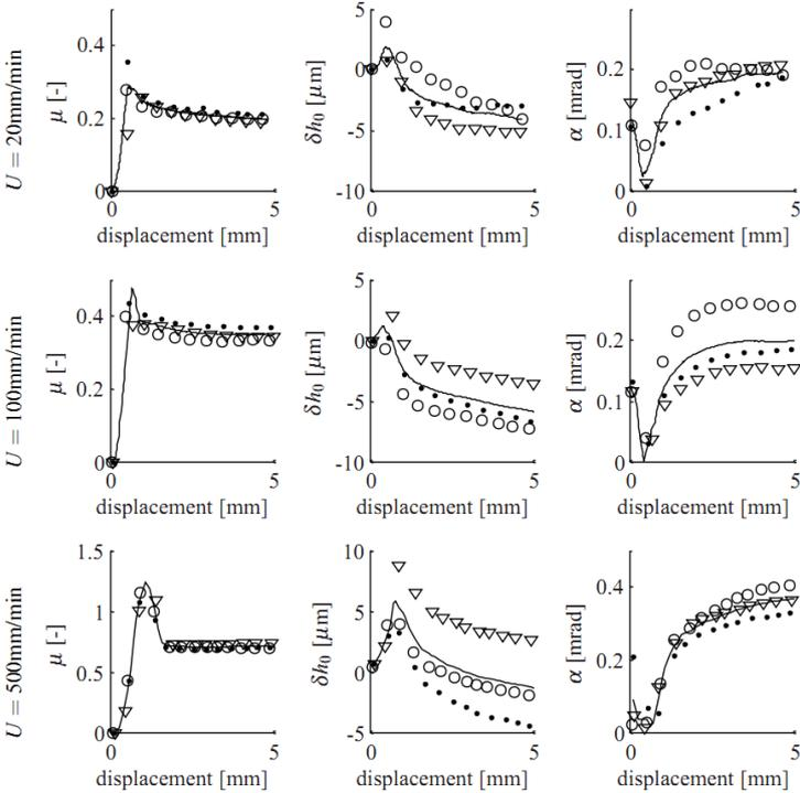
Figure 5: Measurements of (from left to right) friction coefficient, average relative gap and misalignment angle as function of displacement for different pulling velocities. AS4 carbon fiber / Polyetheretherketone (PEEK) UD tape, fibers aligned to pulling direction,  $T = 400^{\circ}\text{C}$  and  $p = 50\text{kPa}$ .
