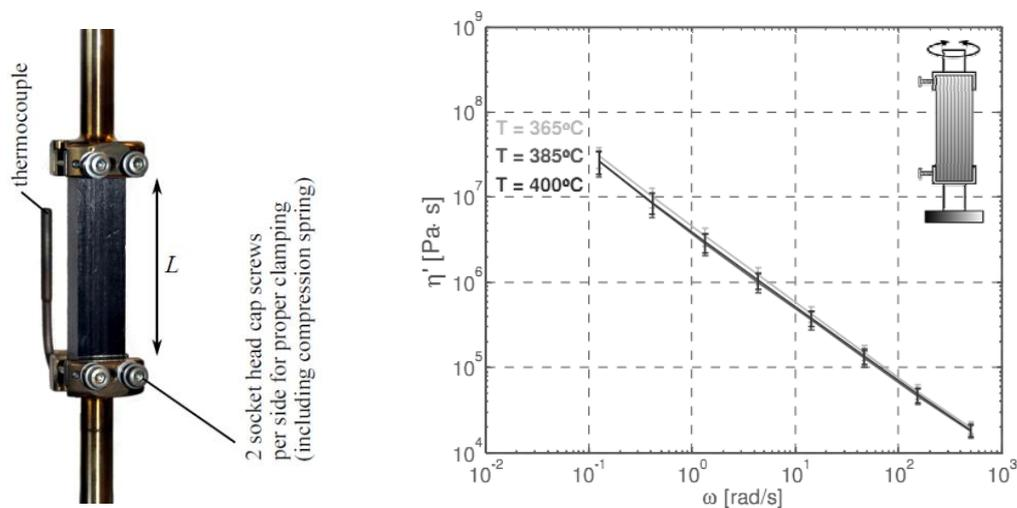
Figure 3: Torsion beam set-up for longitudinal shear identification (left); measured dynamic viscosity versus angular frequency (right)
