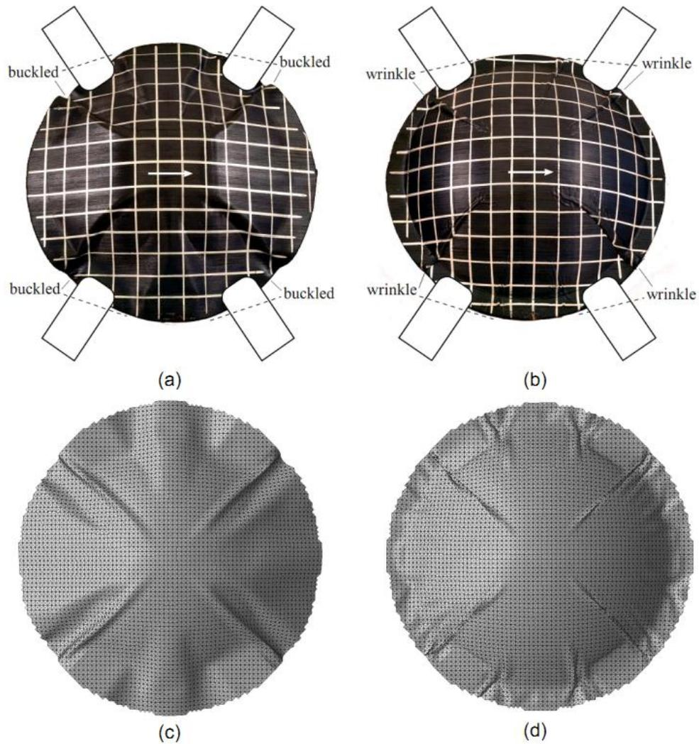
Figure 7: Comparison of experiment (top) and simulation (bottom): intermediate forming result with tool distance of 20mm (a) and final shape (b). Intermediate (c) and final simulation result (d). AS4 carbon fiber /Polyetherketoneketone (PEKK) quasi-isotropic  $[0/90/45/-45]_s$  lay-up
