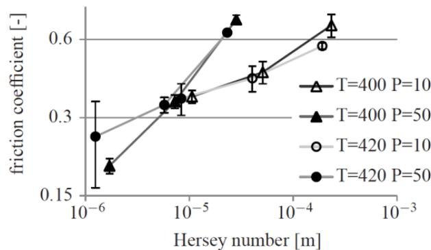
Figure 6: Stribeck curve for steady state friction
