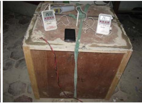
Figure 4.3: Testing of the insulation brick
