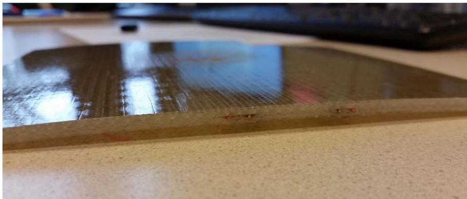
Figure 5: A picture showing the warpage in the co-bonded composite part. The side facing the table is the over infused part.
