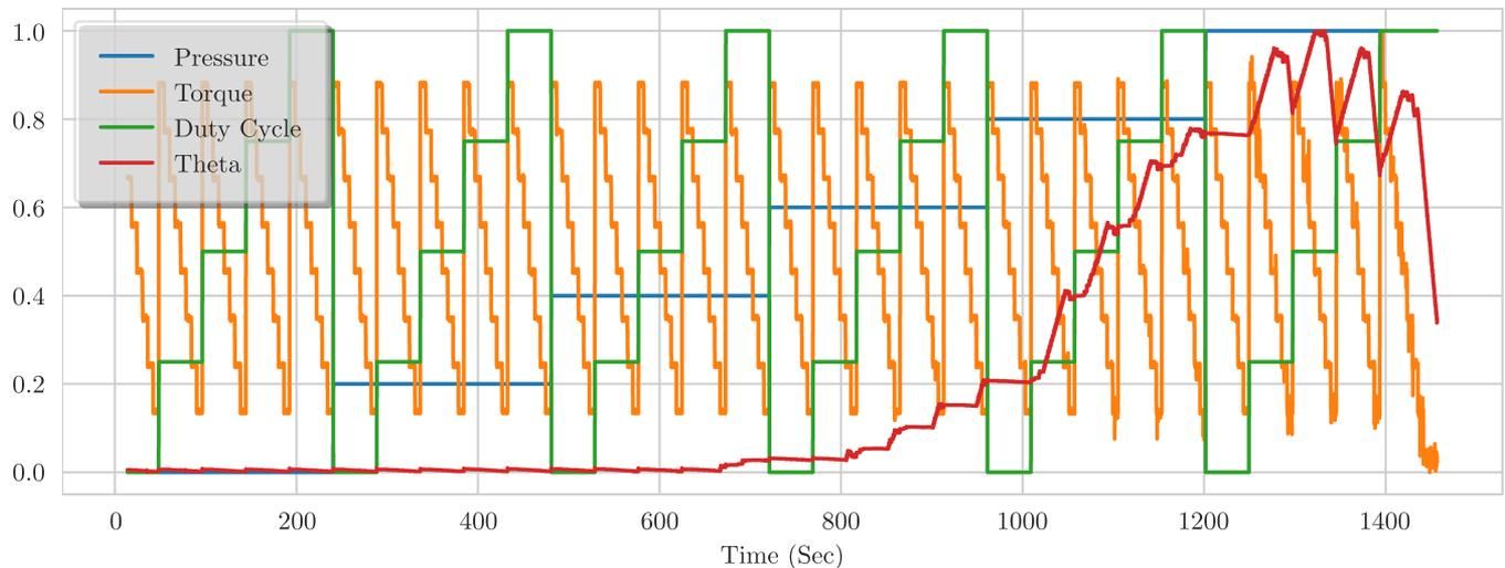
Fig. 9. The stall behavior of a PneuAct-II in Step 1. of Phase 3., in a sample with a clearance of  $224 \mu\text{m}$  at various input pressures, external torques, and duty-cycles is illustrated in a normalized plot. Constant Theta (i.e., position) represent stall of the PneuAct actuator. In certain conditions, especially at high pressures, the PneuAct motor rotates in the opposite direction (i.e., reducing Theta) due to the missing-steps phenomenon, as explained in the text.
