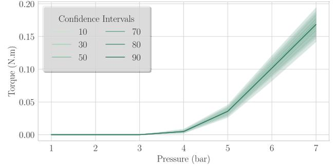
Fig. 5. Bootstrapped stall torque is plotted at various input pressure contoured with different confidence intervals. A linear relationship can be observed as predicted by eq. (1) while an average minimum pressure of 3 bar is required to overcome internal friction and leakage.
