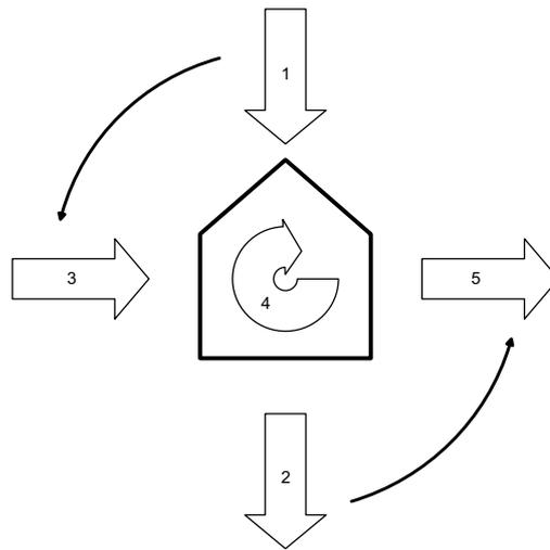
Figure 1: Circular Project Model with large arrows (1-5) representing material flows around a construction project and small arrows indicating a 'transition' from linear to circular practice: 1=new materials; 2=waste; 3=reuse of recovered materials (from an old building); 4=recovery and reuse (from and in the same building); 5=recovery of materials for reuse (in another building)
