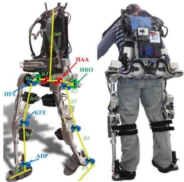
Fig. 3: Exoskeleton developed at University of Twente.
