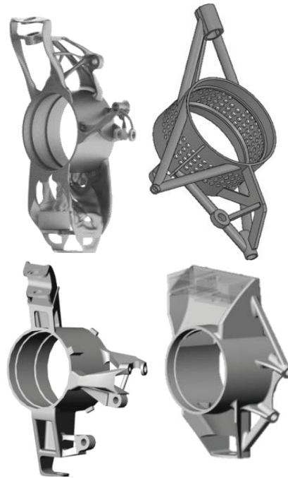
Figure 3 Examples of design strategies as proposed by Lindeman [25]. Top left: CAD remodelling of TO results. Top right: CAD modelling using design rules for AM (no TO). Bottom left: Use of TO and standard CAD features. Bottom right: Combination of TO, CAD features and design rules
