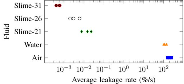
Fig. 1: The average leakage rate of the fluids when pressurized at 550 kPa.
