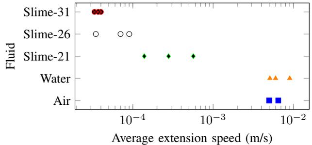
Fig. 2: The average extension speeds of a syringe actuated by the fluids at pressures of 50 kPa (air and water), 100 kPa (Slime-21), and 150 kPa (Slime-26 and Slime-31).
