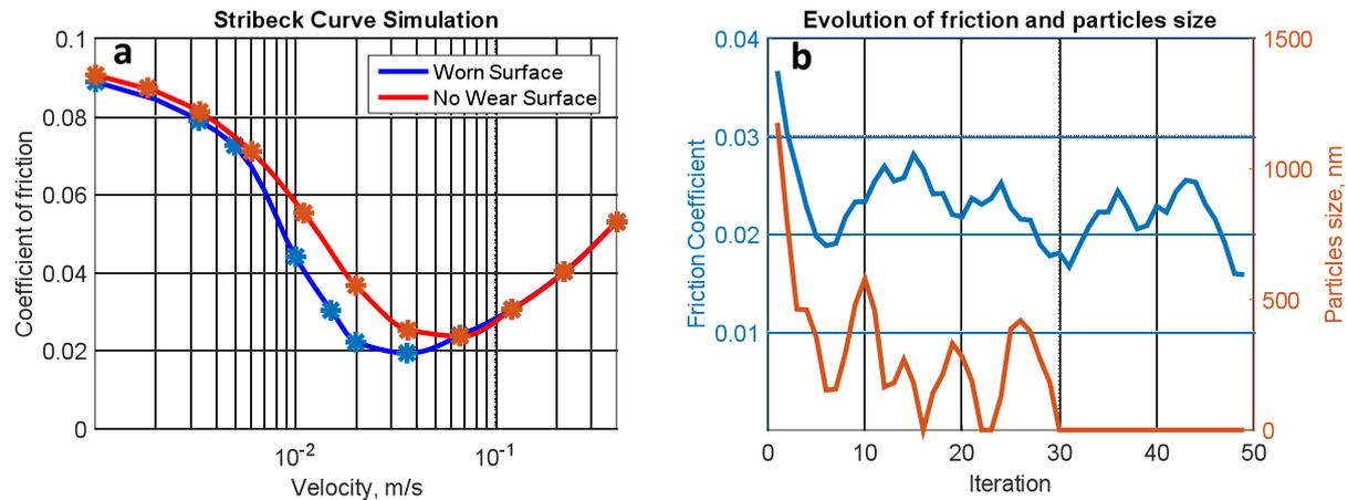
**Fig. 2. Examples showing (a) the effect of wear on friction and (b) evolution of the coefficient of friction and wear particles size at a speed of 0.02/s.**
