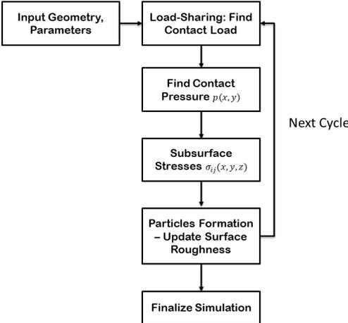
**Fig. 1. The algorithm for particles simulation.**
