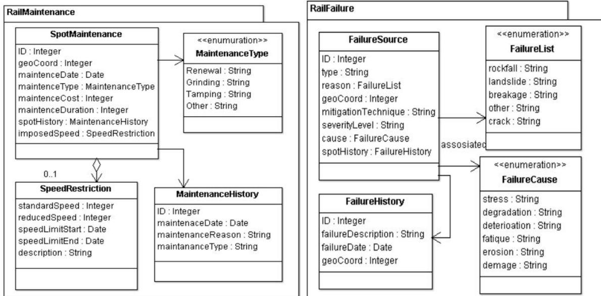
Figure 5: Information Model(Railway Maintenance) Figure 6: Information Model (Railway Failure)
