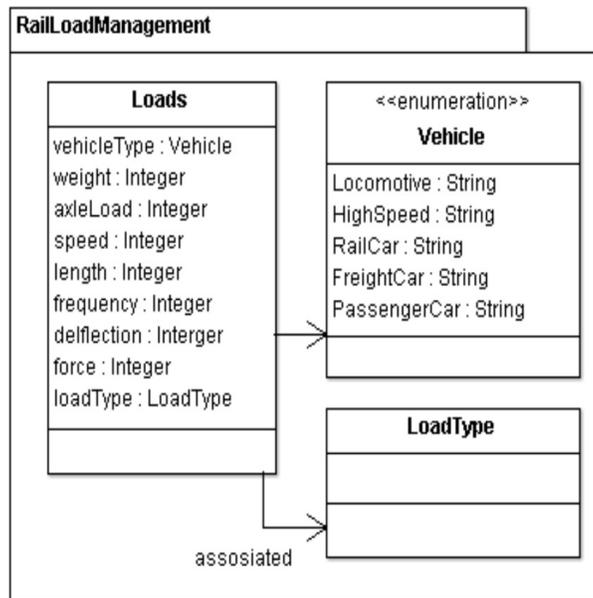
Figure 4: Information Model (Railway Load)
