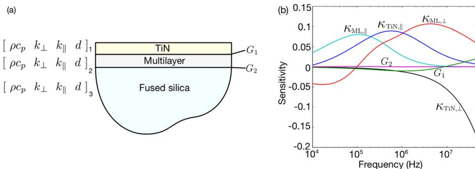
FIG. 2. (a) Sample configuration for FDTR measurements. (b) Calculated phase sensitivity to the cross- and in-plane thermal conductivities of the multilayer,  $k_{ML,\perp}$  and  $k_{ML,\parallel}$ , the cross- and in-plane thermal conductivities of TiN,  $k_{TiN,\perp}$  and  $k_{TiN,\parallel}$ , and the TBCs,  $G_1$  and  $G_2$ .
