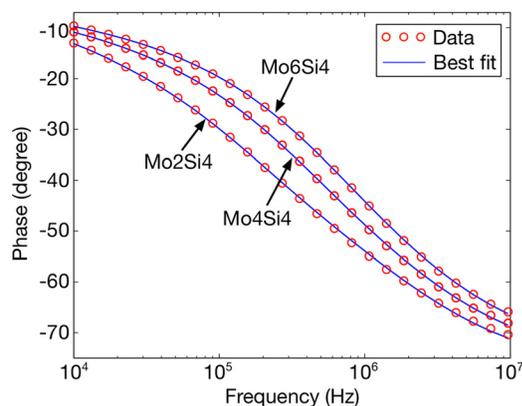
FIG. 3. FDTR measured phase signals and model best fit curves of the three TiN-coated multilayer samples.
