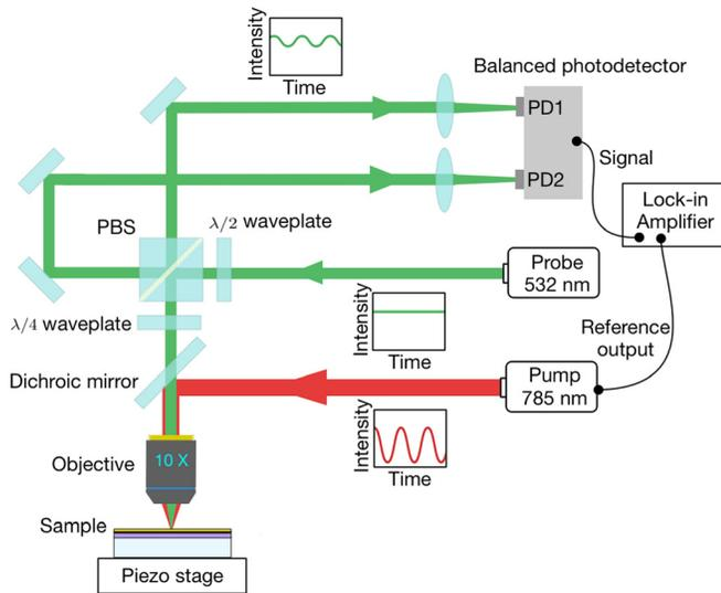
FIG. 1. Schematic of our FDTR microscope. A digitally modulated pump laser heats the sample while a probe beam monitors the surface reflectivity. A balanced photo detector is used to improve the signal to noise ratio.
