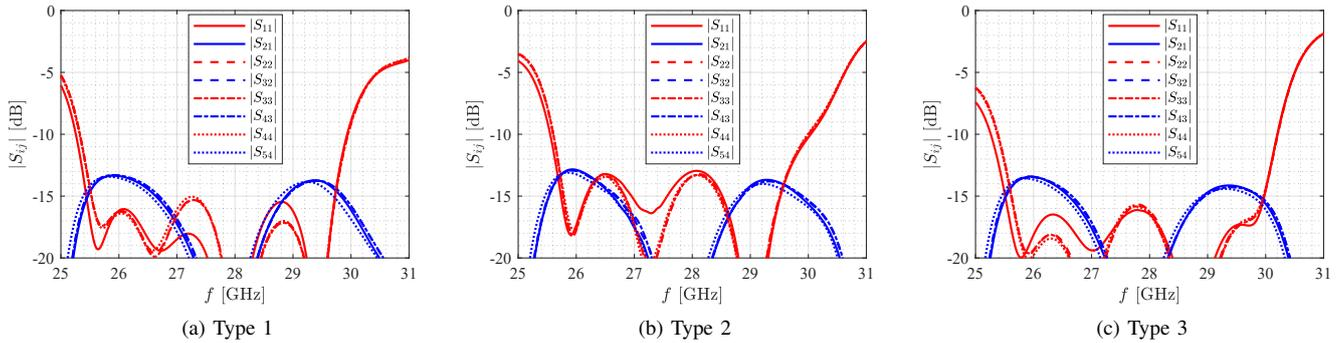
Fig. 4. Reflection coefficient and coupling coefficients with neighbor ports in the array, when the transitions are used to excite the antenna.
