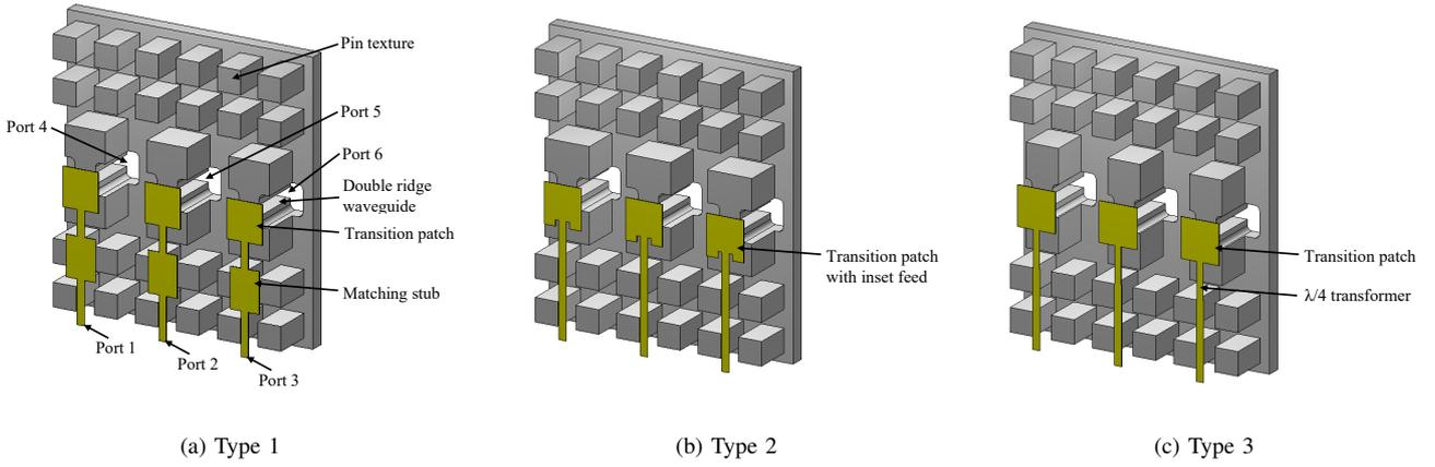
Fig. 1. The structure of three microstrip to double ridge waveguide transitions. In these figures, substrate and ground layer of microstrip lines are not shown.
