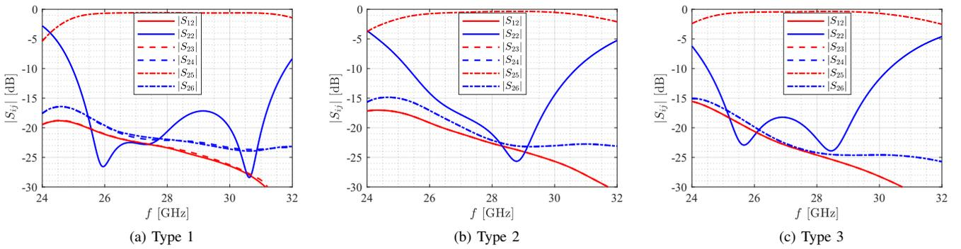
Fig. 2. Scattering parameters of each transition.
