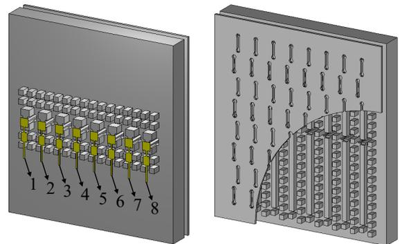
Fig. 3. Integration of transition type 1 with a 5G antenna array based on gap waveguide technology [9]. A part of slot layer is cut for viewing purposes. The number of port for each microstrip line is shown in left side picture.
