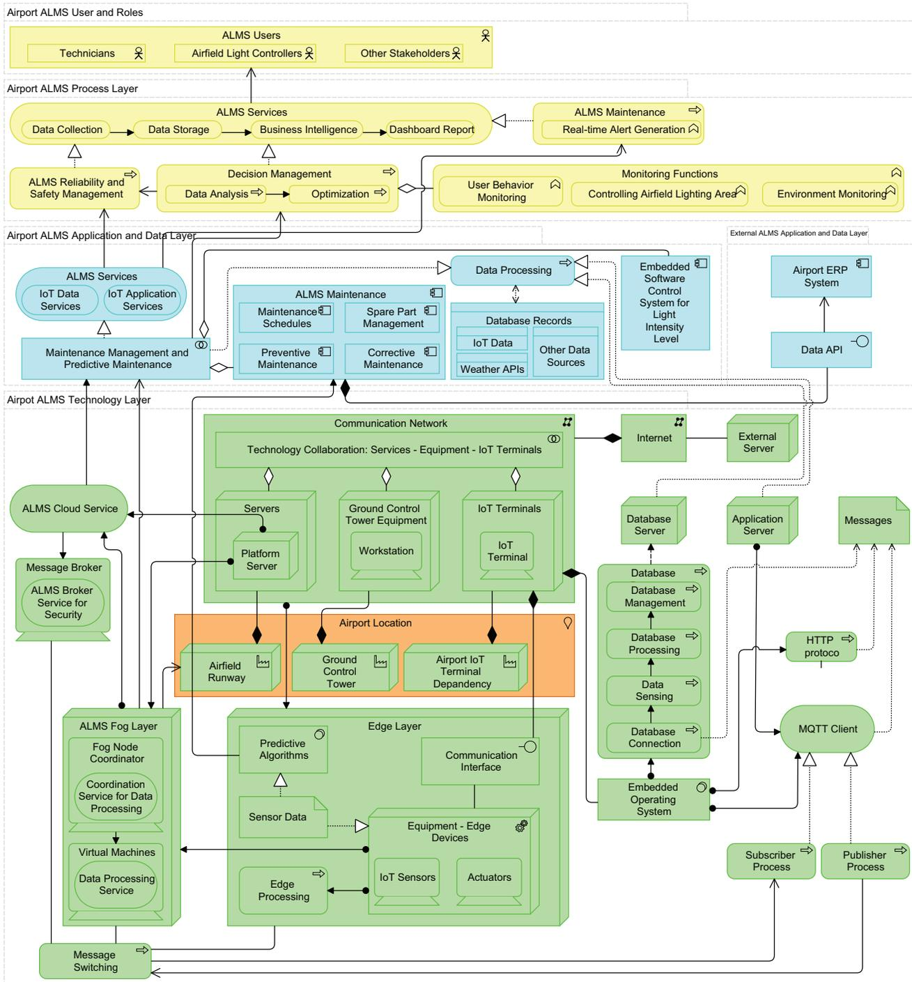
Fig. 8. Enterprise Architecture - ALMS Based on IoT
