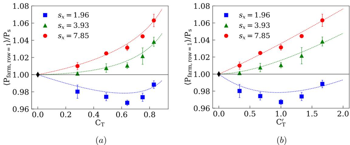
**Figure 4.** The power output for the average turbine in the first row of a wind farm with  $s_y = 1.57$  and different streamwise spacings ( $s_x$ ) is compared to that of a free-standing turbine as a function of a)  $C_T$  and b)  $C'_T$ . The dashed lines are calculated from the fits obtained in Figures 2 and 3.
