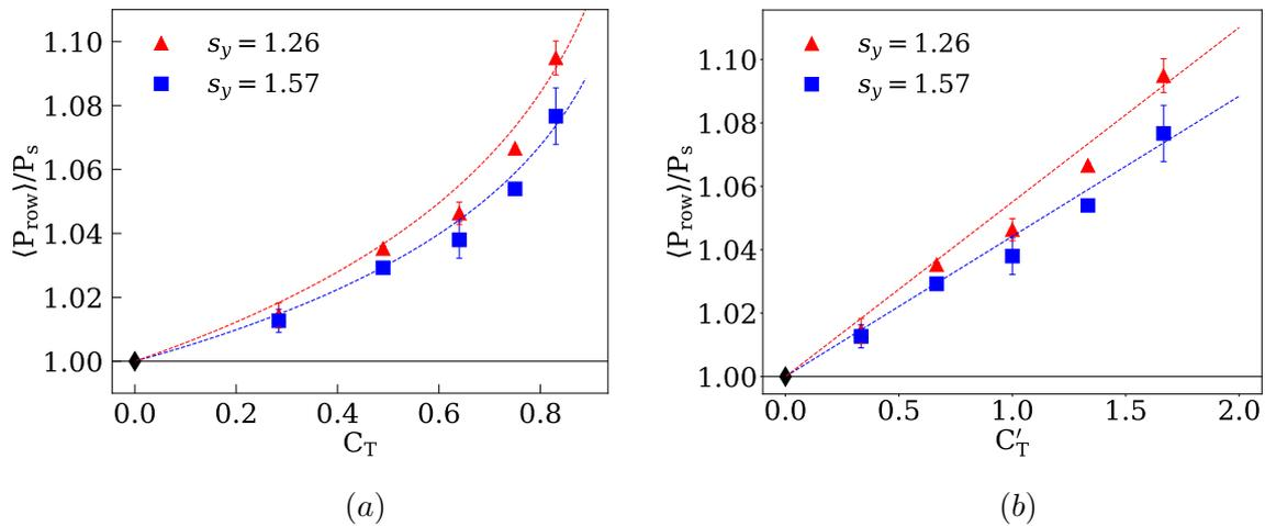
**Figure 2.** The average power output of a turbine in an infinite, closely-spaced ( $s_y$ ) row relative to the average power output of a free-standing turbine as a function of a)  $C_T$  and b)  $C'_T$ . The dashed lines indicate the least-squares fit to the  $\langle P_{\text{row}} \rangle / P_s$  versus  $C'_T$  data in the right figure. The corresponding lines in the left figure are obtained using Equation 4.
