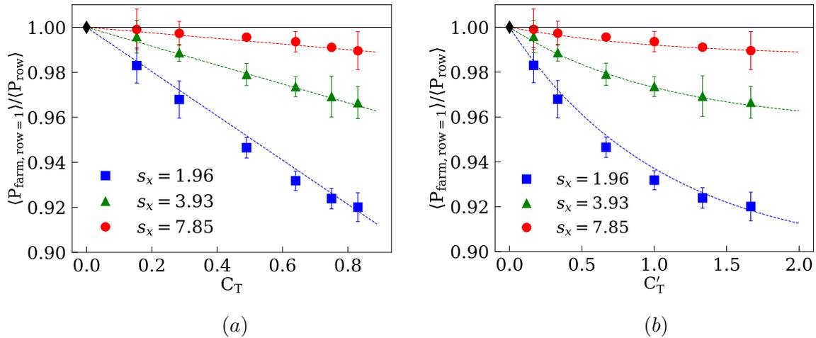
**Figure 3.** The power output for the average turbine in the first row of a wind farm with  $s_y = 1.57$  and different streamwise spacings ( $s_x$ ) is compared to that of a solitary, infinite row as a function of a)  $C_T$  and b)  $C'_T$ . The dashed lines indicate the least-squares fit to the  $\langle P_{\text{farm, row}=1} \rangle / \langle P_{\text{row}} \rangle$  versus  $C_T$  data in the left figure. The corresponding lines in the right figure are obtained using Equation 4.
