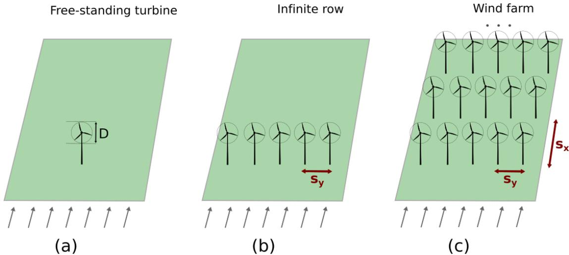
**Figure 1.** Schematic depicting the three main cases considered in this study: (a) a free-standing turbine (b) an infinite row, and (c) a wind farm with eight rows in the downstream direction. The streamwise ( $s_x$ ) and spanwise ( $s_y$ ) spacing are made non-dimensional using the turbine diameter  $D$ , i.e.,  $s_x = S_x/D$ ,  $s_y = S_y/D$ . See Table 1 for a detailed overview of the cases considered.
