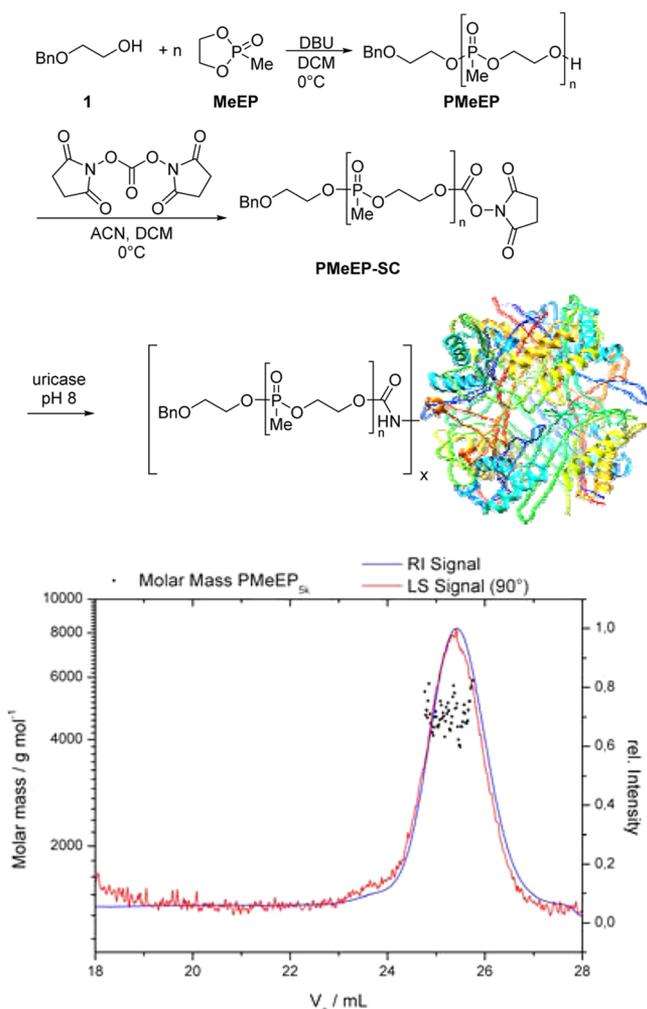
**Figure 1.** (a) Polymerization of MeEP and  $\omega$ -postmodification with DSC yielding amino-reactive PMeEP-SC. (b) MALLS-SEC analysis of PMeEP indicating a narrow molecular weight distribution and a molecular weight close to  $5000 \text{ g mol}^{-1}$ .
