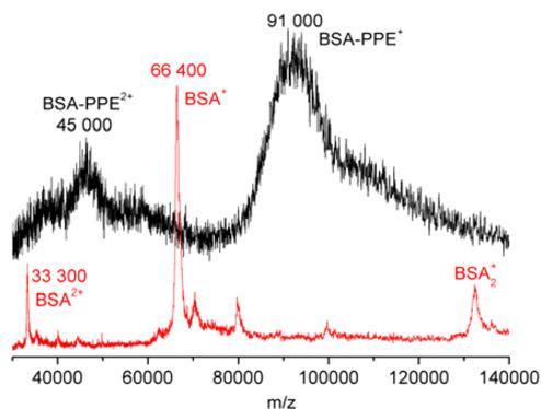
**Figure 3.** MALDI-ToF MS of unmodified BSA (red) and BSA-PPE conjugate (black). Increasing  $m/z$  indicates successful bioconjugation, confirming SEC-MALLS measurements.
