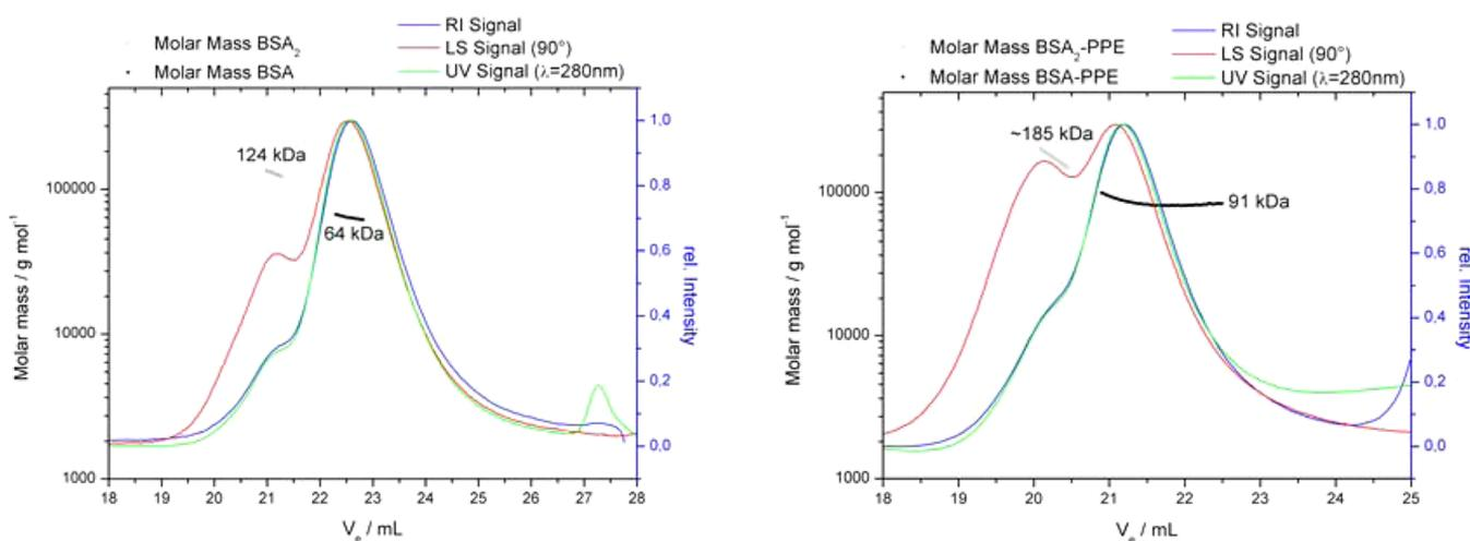
**Figure 2.** Aqueous SEC traces of BSA (*left*) and the BSA-PPE conjugate (*right*) measured by triple detection (refractive index, light scattering, UV). The molecular weight calculated from LS and RI data is given for the homodimer (124 kDa) and homomonomer (64 kDa) of BSA. After conjugation the molecular weight increases for both species to 185 kDa and 91 kDa, respectively.
