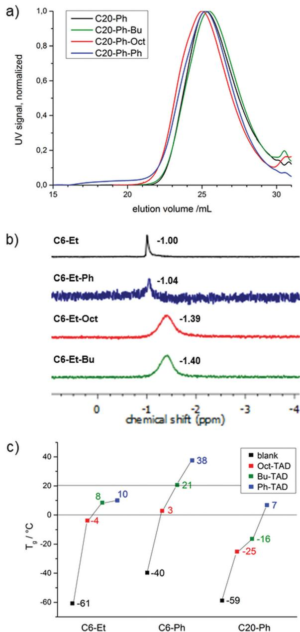
Fig. 2 (a) SEC traces of C20-Ph, C20-Ph-Bu, C20-Ph-Oct and C20-Ph-Ph in THF, UV signal; (b) <sup>31</sup>P-NMR spectra of C6-Et, C6-Et-Bu, C6-Et-Oct and C6-Et-Ph; (c) T<sub>g</sub>'s of all PPEs.
