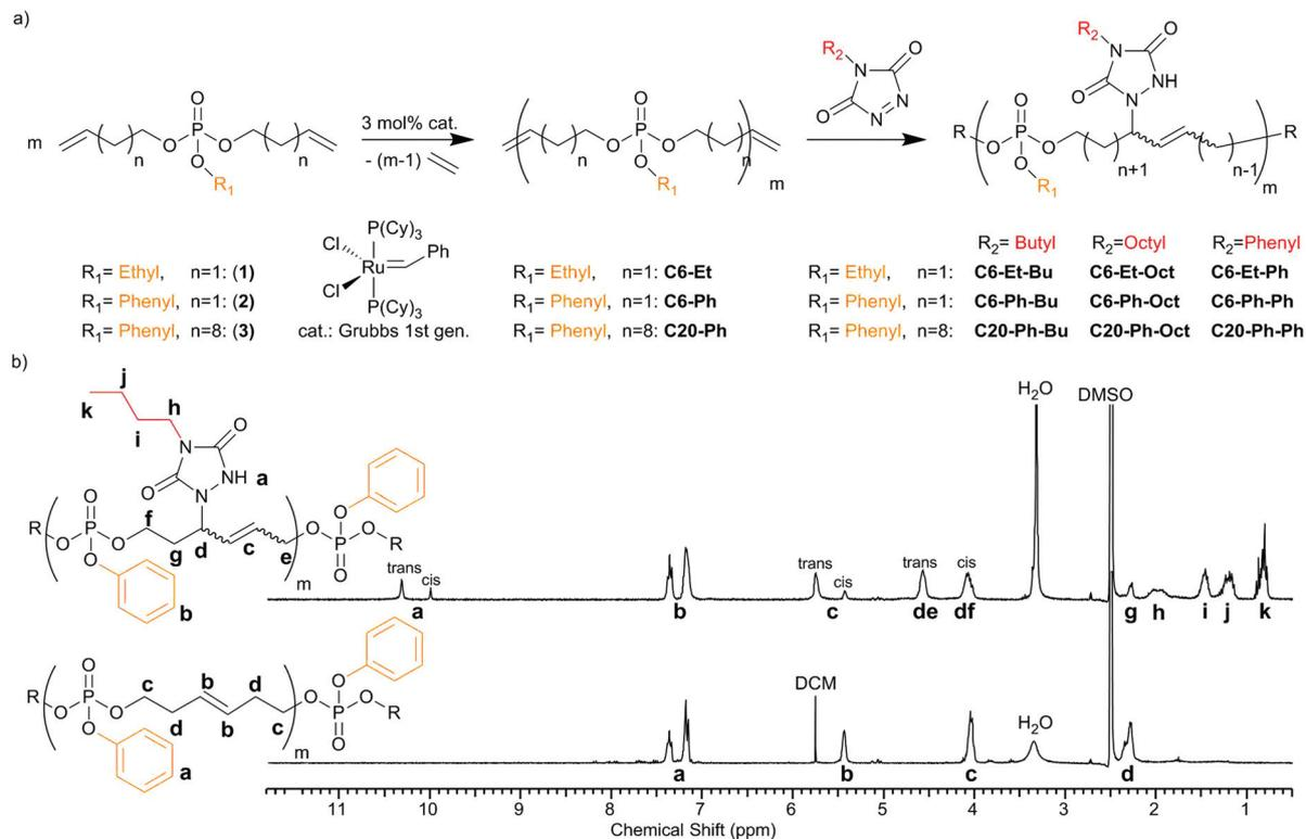
**Fig. 1** (a) Synthesis scheme of C6-Et, C6-Ph and C20-Ph and post-modification with Bu-TAD, Oct-TAD or Ph-TAD; (b)  $^1\text{H}$  NMR spectra of polymers C6-Ph (bottom) and C6-Ph-Bu (top) (300 MHz, 298 K, DMSO- $d_6$ ).
