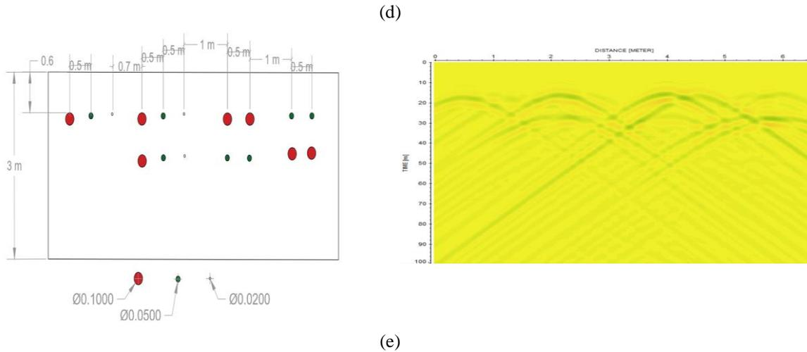
Figure 4. First group pipes cross-section (left) and related radargram (right)
