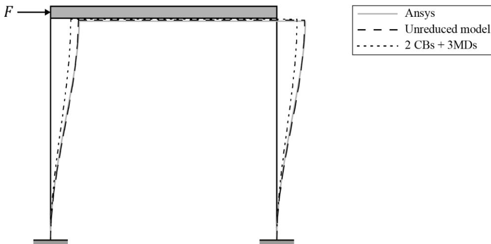
Figure 4: Equilibrium analysis of a parallel leaf spring mechanism subjected to a horizontal load
