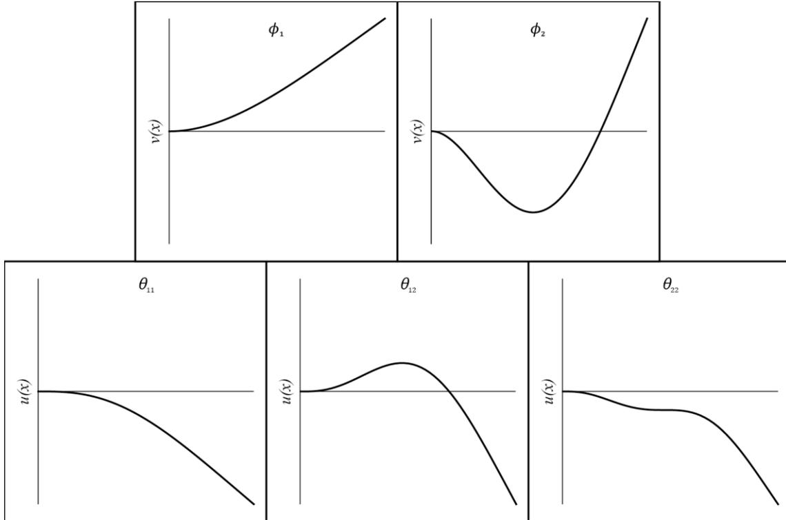
Figure 1: Vibration modes and modal derivatives of a cantilever beam
