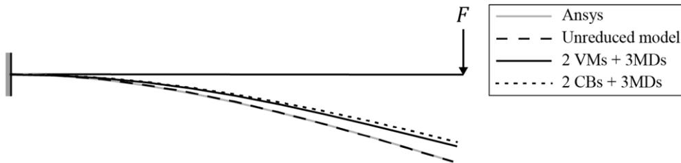
Figure 3: Equilibrium analysis of a cantilever beam subjected to a tip load
