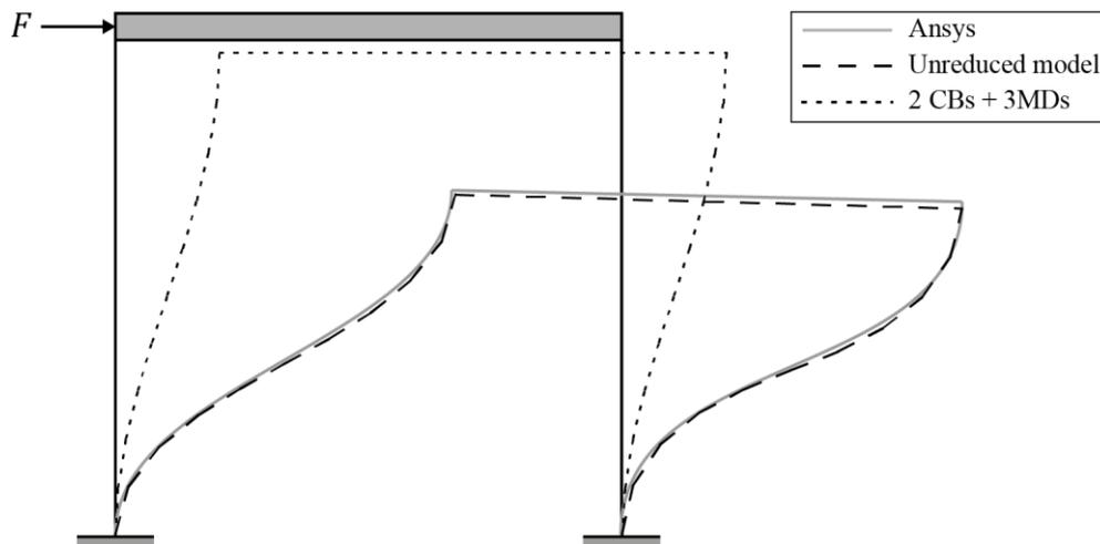
Figure 6: Equilibrium analysis of a parallel leaf spring mechanism subjected to an increased load
