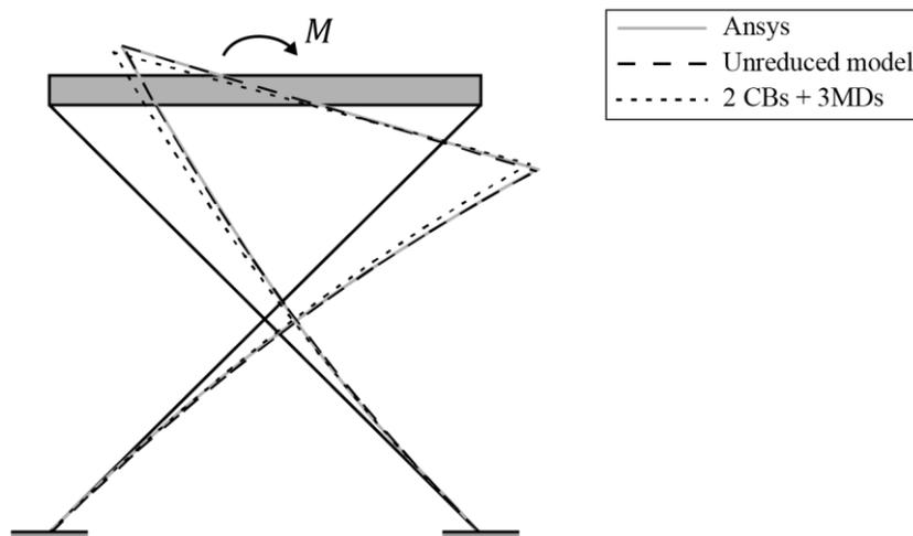
Figure 5: Equilibrium analysis of a cross flexure mechanism subjected to a bending moment
