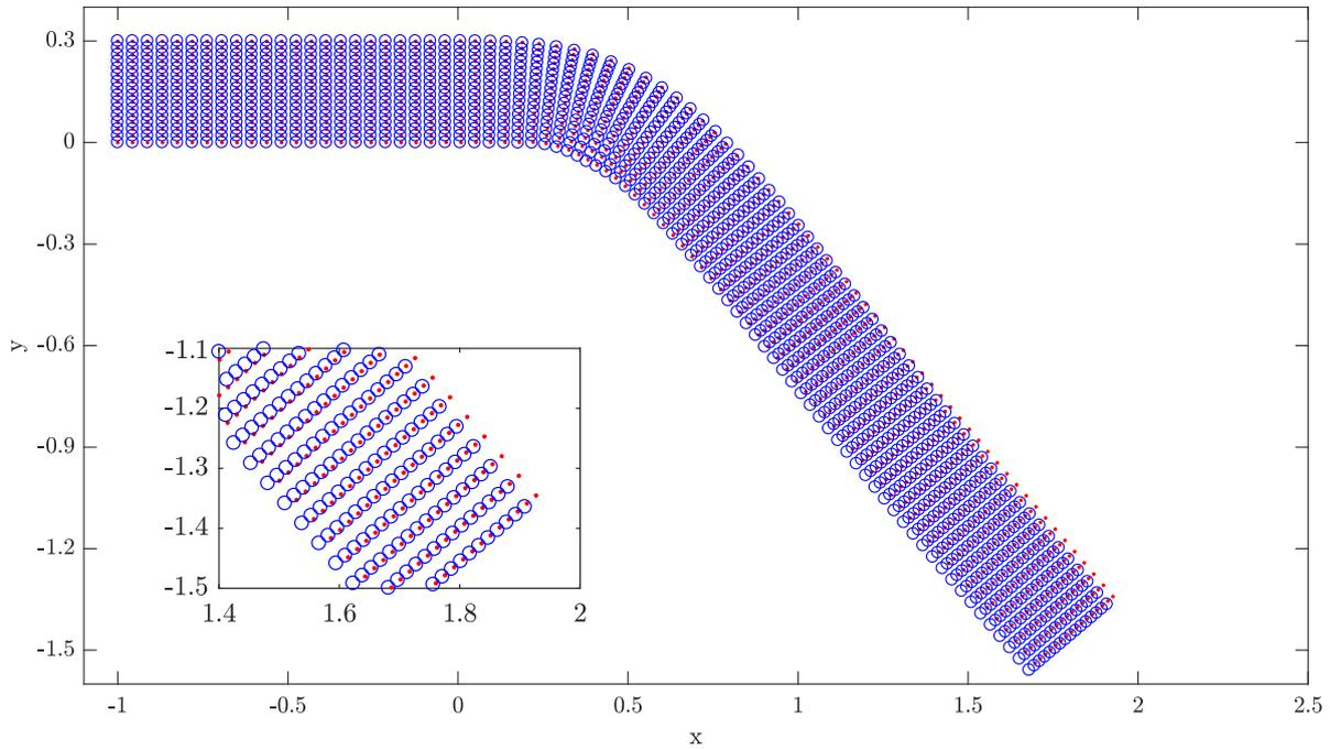
Figure 4: Output of the displacement field  $\{\mathbf{u}, \mathbf{v}\}$  from both the first stage SVD MQ-RBF metamodel ( $\cdot$ ) and the FE model ( $\circ$ ). The zoomed panel shows the region with the largest RMSE.
