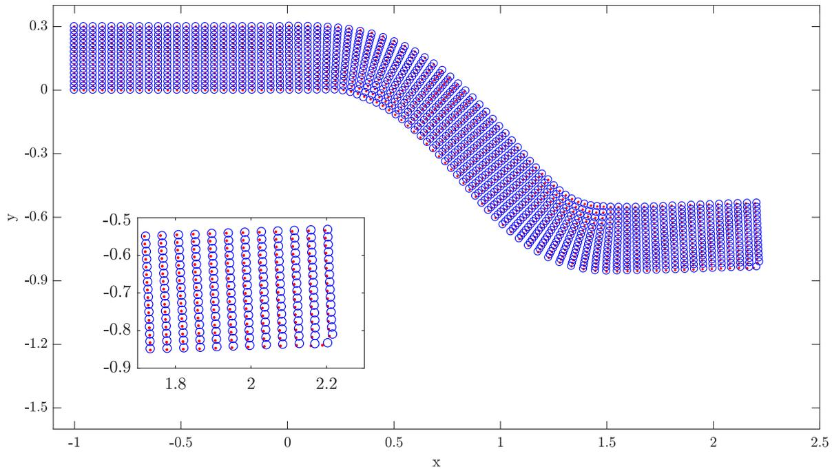
Figure 5: Output of the displacement field  $\{\mathbf{u}, \mathbf{v}\}$  from both the first stage SVD MQ-RBF metamodel combined with the second stage FE model ( $\cdot$ ) and when both stages are modeled using the FE model ( $\circ$ ). The zoomed panel shows the region with the largest RMSE.
