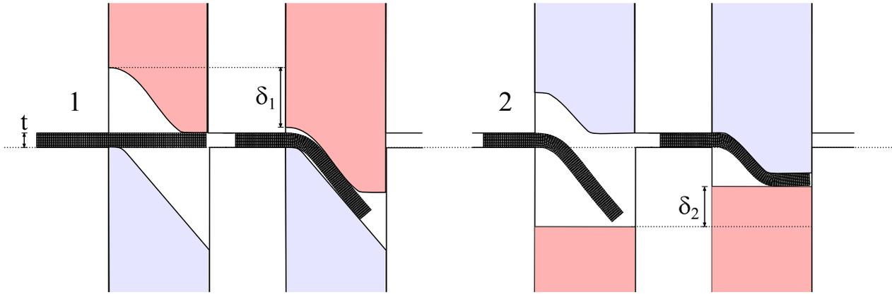
Figure 2: Schematic representation of the two stage FE model.
