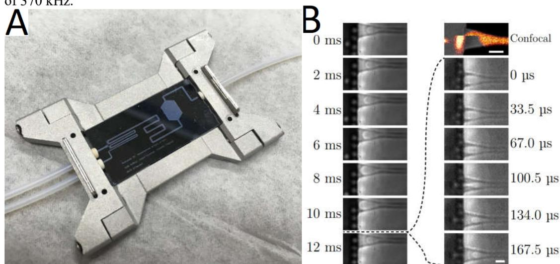
Figure 2: A) The glass/silicon Nanopede chip in the redesigned chip holder. Due to the removal of excess material on the side of the chip, high magnification lenses can reach the chip and image the nanoscale nozzles. B) The droplet production mechanism of the Nanopede. The left column shows the full formation cycle of one droplet, while the right column shows the moment of release at  $3 \times 10^4$  frames per second. Images were procured using a full glass chip.
