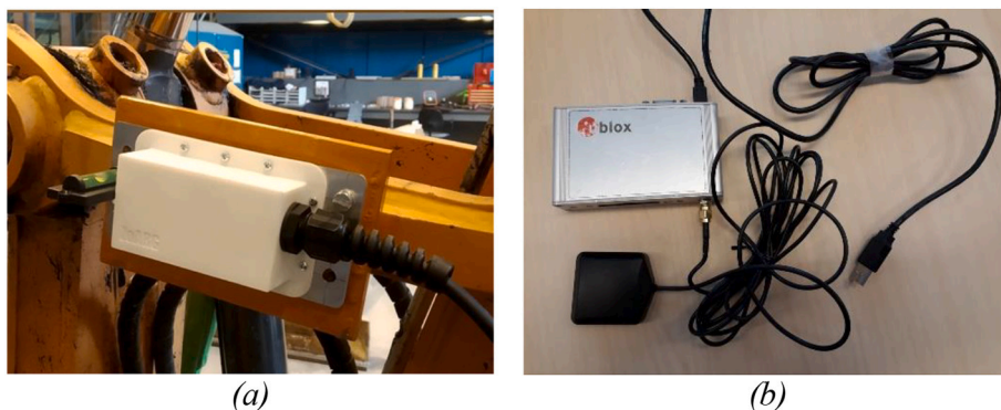
Fig. 7. (a) IMU for pose estimation and (b) GNSS for localization.
