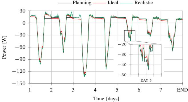
Fig. 4. Power profile of the neighborhood of 10 scaled households including the planning for the realistic battery model case.
