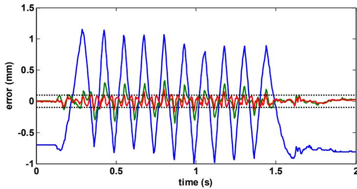
Figure 2: The tracking error without ILC (blue), in the third iteration of ILC using an LTI model (green) and using an LTV model (red).
