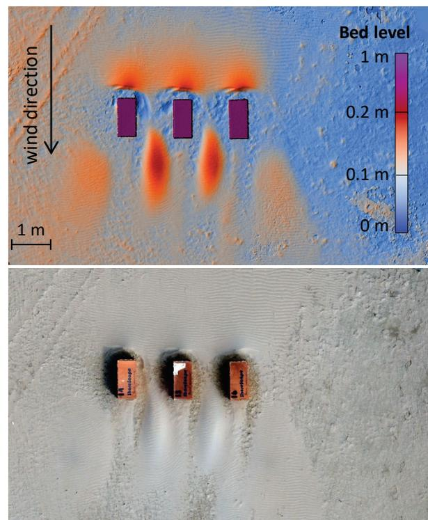
Figure 2 - A DEM (top) and orthophoto (bottom) of the deposition around a row of 3 boxes (size 1x0.5x0.5m)
