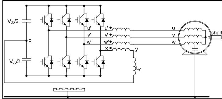
**Figure 4.** The diagram of the fourth leg approach
