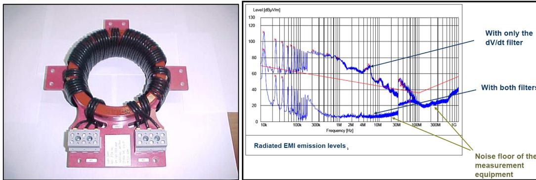
**Figure 3:** Final common mode choke with nanocrystalline material and final radiated emission level of the overall filter
