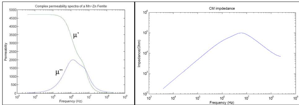
**Figure 1:** Complex permeability spectrum of a Sintered MnZn ferrite and its common mode impedance (Dimension: 25\*10\*5 mm, N=20)
