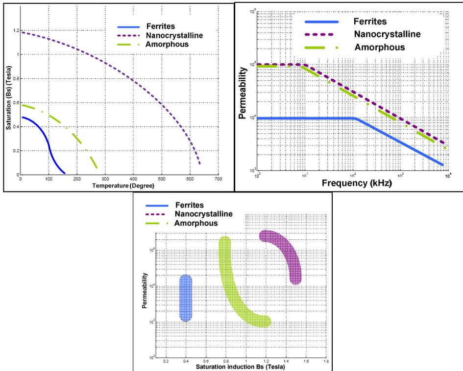
**Figure 2:** Main magnetic properties for the material ferrites, nanocrystalline and amorphous: Saturation vs. Temperature, Permeability vs. Frequency, and Saturation vs. permeability
