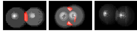
Fig. 4: Erroneous peaks (red) in Hough Transform for pitch (left) and yaw (center), are suppressed by element-wise multiplication.
