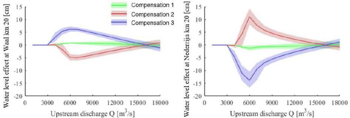
Figure 2: Effects on water levels at locations downstream of the interventions in the Waal (left) and Nederrijn (right) branch caused by the 3 variations of compensating interventions (see Table 1). The continuous line marks the mean effect and the shaded area marks the 90% confidence interval.
