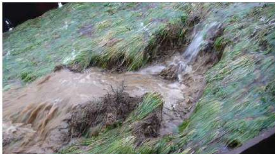
Figure 1: Erosion of the grass cover by overtopping waves results in the formation of a small cliff (Peeters et al., 2012).
