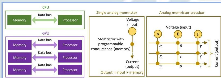
Fig. 1 The computing process in CPU, GPU and memristors.<sup>2</sup>
