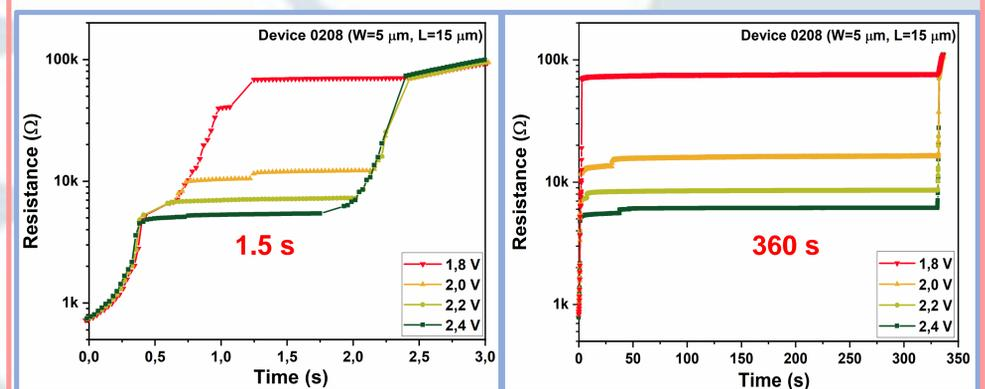
Fig. 6 Stable resistive states under different voltage bias.
