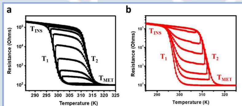
Fig. 2 Temperature-dependent resistivity of VO<sub>2</sub> film.<sup>3</sup>
