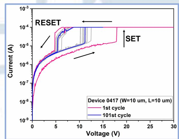
Fig. 4 Voltage linear sweep for 101 cycles.
