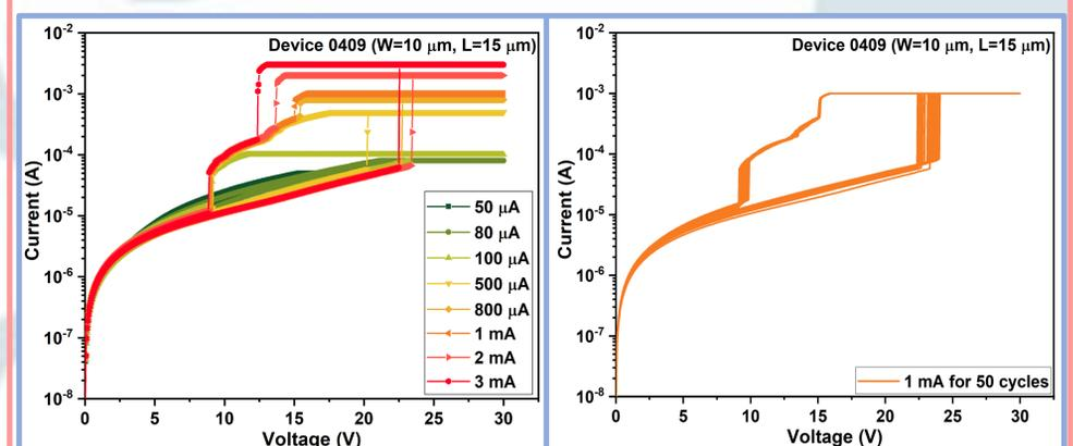
Fig. 5 Left Voltage linear sweep with different compliances. Right Voltage linear sweep with compliance at 1 mA for 50 cycles.
