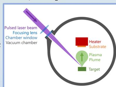
Fig. 3 Schematic of PLD.
