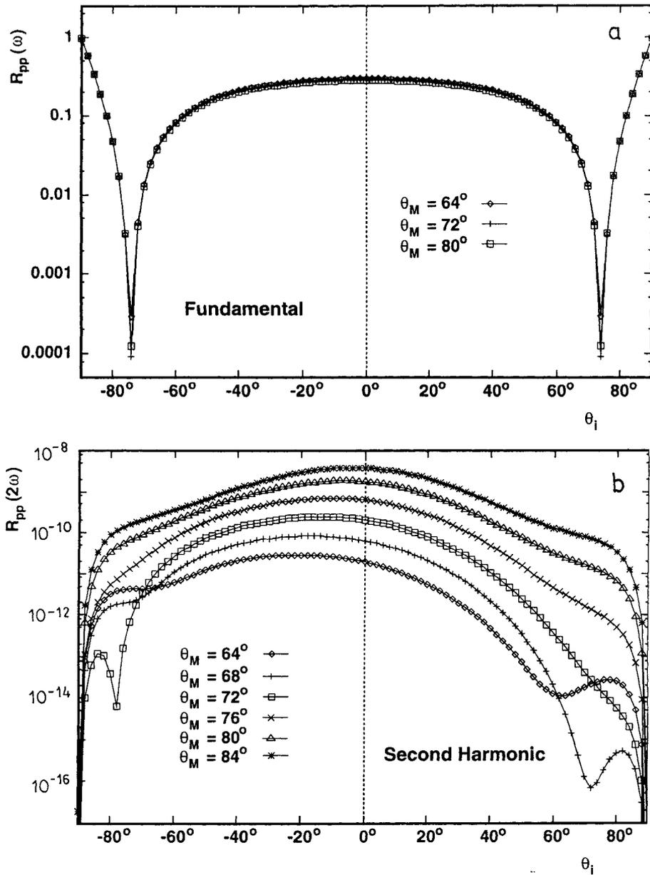
Fig. 3. pp-type reflectance as a function of  $\theta_i$  for  $\Omega = 0^\circ$  and 48 layers of calix at several high values of  $\theta_M$
