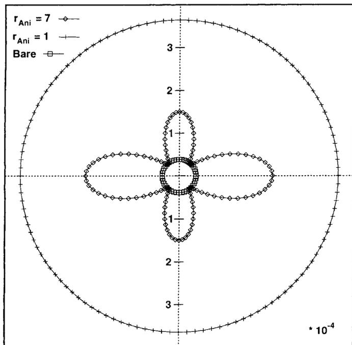
Fig. 6. pp-type reflectance as a function of  $\Omega$  for  $\theta_i = 74^\circ$ ,  $\theta_M = 84^\circ$ . Bare Si, 48 layers  $r_{\text{Ani}} = 1.0$ , and 48 layers  $r_{\text{Ani}} = 7.0$
