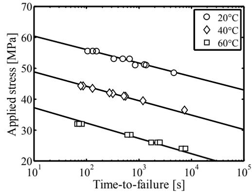
Figure 2: Time-to-failure for a range of applied stresses and temperatures.
