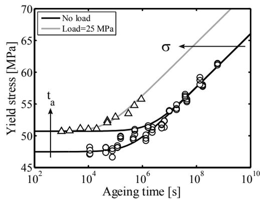
Figure 3: Master curve constructed using time-temperature superposition on experimental yield data (circles) and the influence of applied load and initial age.
