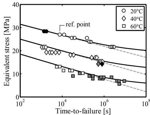
Figure 3: Failure times burst tests on uPVC pipes, reproduced from [5]. The unfilled, grey and black markers represent ductile tearing, hairline cracking and brittle fracture respectively. The lines are model predictions.
