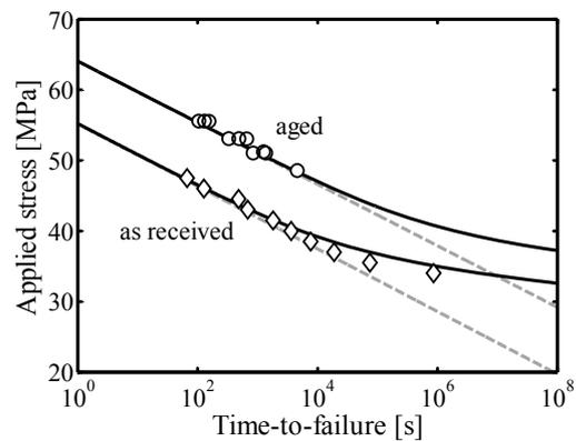
Figure 4: Time-to-failure for tensile bars under constant uni-axial tensile stress. The markers are experimentally obtained values, the lines are model predictions.
