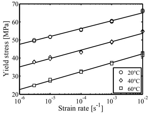
Figure 1: Tensile yield stress data for a range of strain rates and temperatures.
