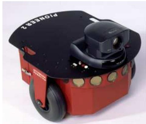
Figure 1: A pioneer 2 DX robot with camera.
