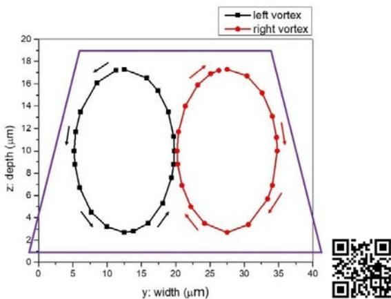
Figure 4. Schematic shape of counter rotating vortices for rectangular shape with imperfect corners, (effectively creating a trapezoid) and a QR code of the experimental recording. Particle focusing at the stagnation point between the vortices was previously reported ( $\mu$ TAS, Taiwan 2018).
