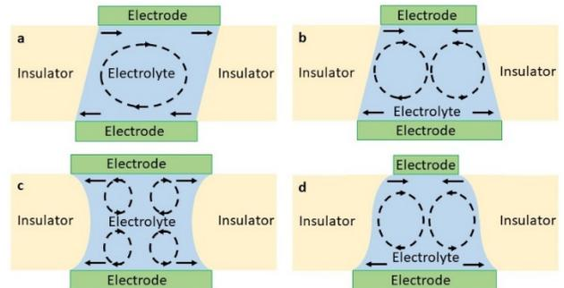
Figure 2. Several channel shapes and the EOF direction at each corner based on the theory of Figure 1.
