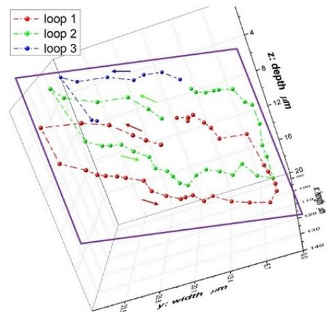
Figure 5. Melamine resin particle (0.5 μm diameter) trajectory in parallelogram-shaped microfluidic device. 2 V peak-peak applied potential and 1 kHz frequency.
