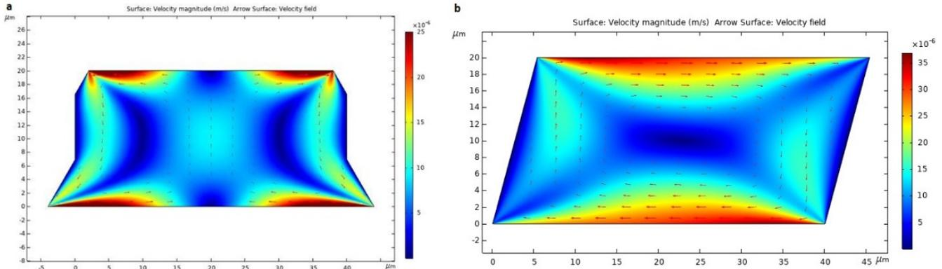
Figure 3. 2-dimensional COMSOL simulations of AC-EOF a) for rectangular shape with imperfect corners and b) for a parallelogram shape, both with a potential amplitude of 0.5 V peak-peak.
