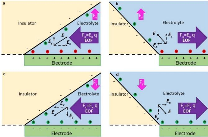
Figure 1. AC-EOF direction a) and c) for sharp corner and opposite polarities. b) and d) For obtuse corner and opposite polarities. For full cycle,  $F_y=0$ .
