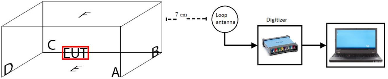
Fig. 1: Measurement setup with specifications of positions around the EMI
