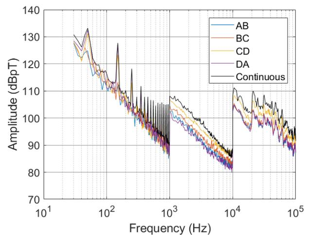
Fig. 7: Comparison of the magnetic field emission at four positions with the worst case scenario over all positions around the EMI
