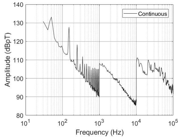
Fig. 6: Worst case magnetic field emission over all positions
