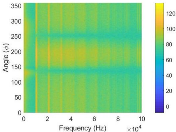
Fig. 5: Magnetic field emission over frequency and position in a circle around the EMI
