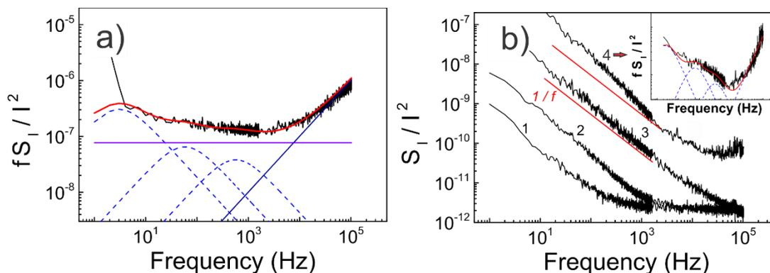
Fig. 1 a) Normalized current noise spectral density, measured for Au NWs with oleylamine molecules; b) Noise spectral density measured for bare Au NWs with diameters in the range of 2 nm to 5 nm (curves 1–3) and for 5 nm diameter Au NW with oleylamine deposited on the nanowire surface (curve 4). For clarity, curve 4 is replotted in the inset. Two well-resolved Lorentzian-shaped components at characteristic frequencies of 3 Hz and 58 Hz are related to molecule-nanowire interactions.
