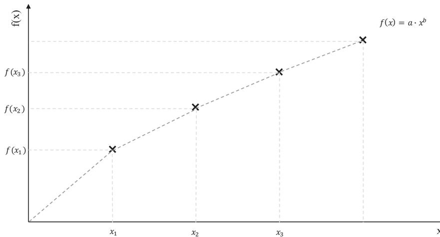
Fig. 3. Example of Piece-wise linearized function.
