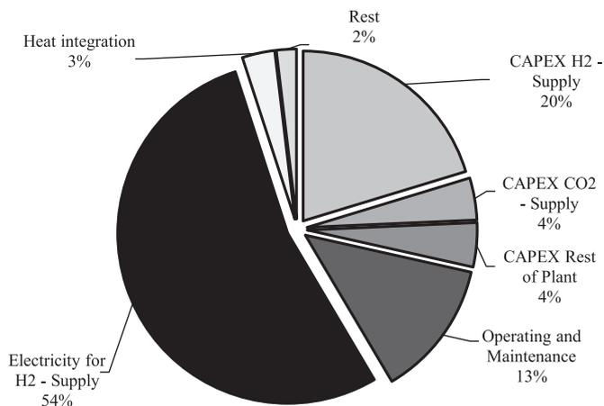
Fig. 6. Cost Breakdown of cost optimal Power-to-Methanol Case.
