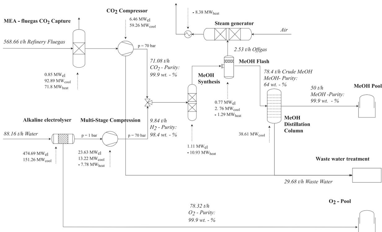
**Fig. 5.** Process flow-sheet of cost-optimized Power-to-Methanol process.
