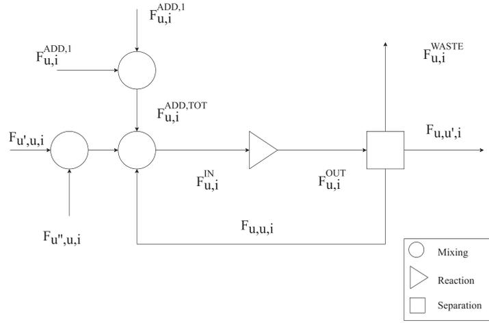
Fig. 1. Mass balance concept for a generic unit-operation  $u \in U$  (e.g. a stoichiometric/ yield reactor or stream splitter).
