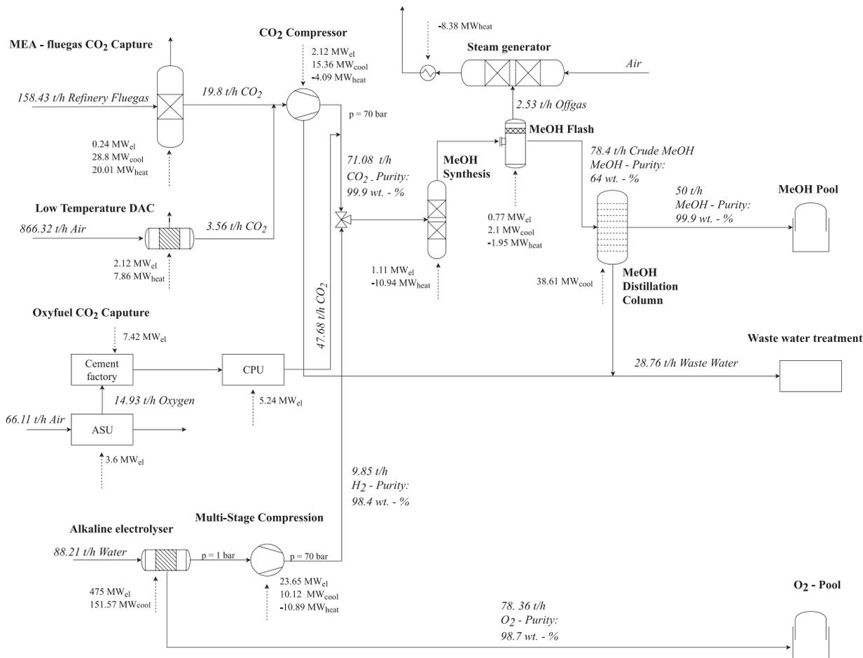
Fig. 7. Process flowsheet of the environmentally optimized Power-to-Methanol process.
