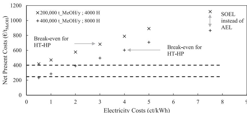
Fig. 9. Sensitivity analysis of net present costs of methanol based on electricity prices and plant capacity (dotted lines represent conventional methanol prices).
