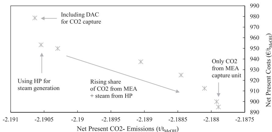
Fig. 8. Pareto-front of Power-to-Methanol optimization.
