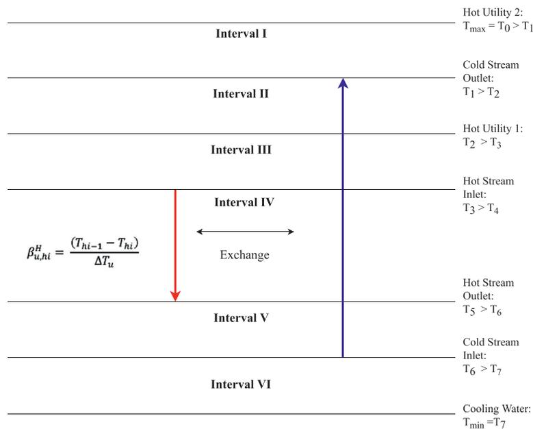
Fig. 2. Example representation of the temperature grid with heat intervals.
