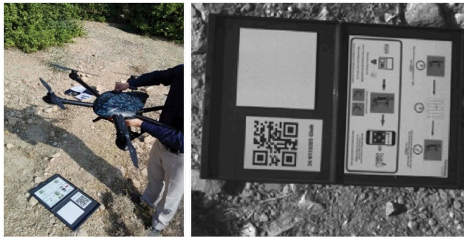
Figure 7. Left: reflectance panel image acquisition, right: Red edge band captured from reflectance panel.
