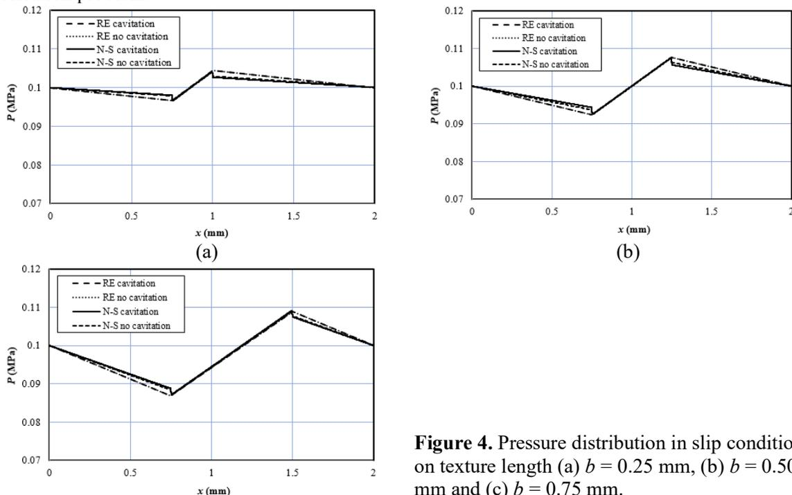
Figure 4. Pressure distribution in slip condition on texture length (a)  $b = 0.25$  mm, (b)  $b = 0.50$  mm and (c)  $b = 0.75$  mm.
