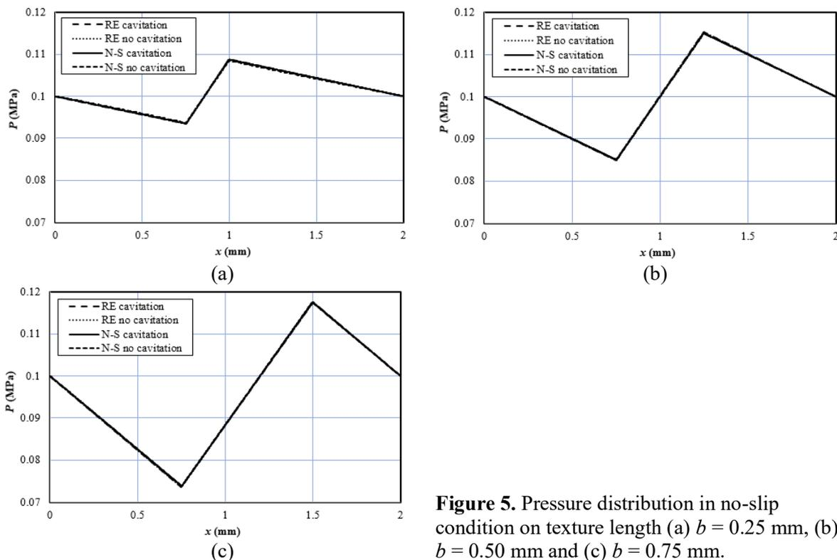
**Figure 5.** Pressure distribution in no-slip condition on texture length (a)  $b = 0.25$  mm, (b)  $b = 0.50$  mm and (c)  $b = 0.75$  mm.
