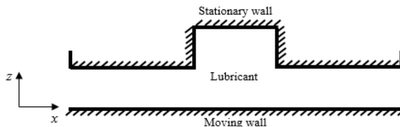
Figure 1. Model of two-dimensional slider bearing.
