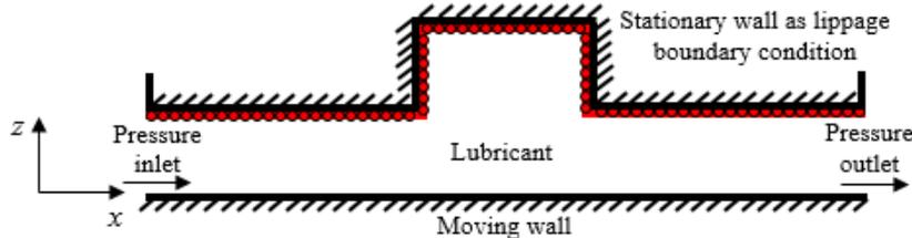
Figure 3. Slippage boundary condition of two-dimensional slider bearing.
