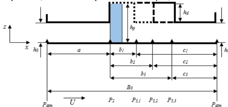
**Figure 2.** Geometry of two-dimensional slider bearing.
