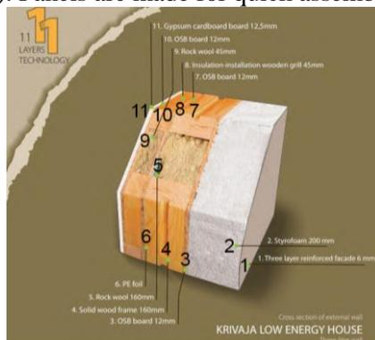
1. Three layer reinforced façade 6mm
