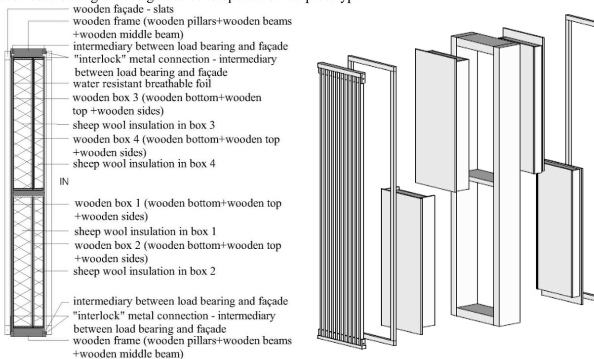
**Figure 2.** Façade system made of wood developed for Green Design Center in Mostar [4], [5]
