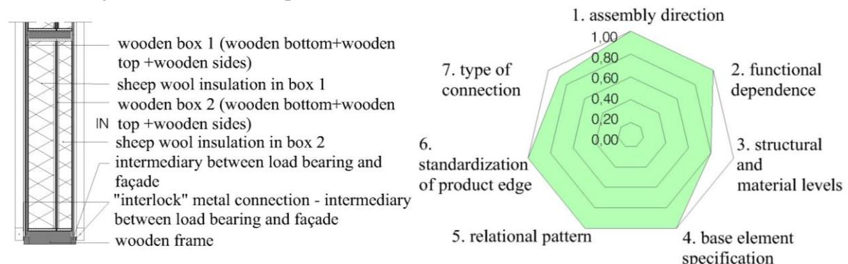
**Figure 4.** The section (left) and the overview of main criteria of reversibility and final score of the reuse potential of a GDC wall -developed façade system (right) using method Durmisevic
