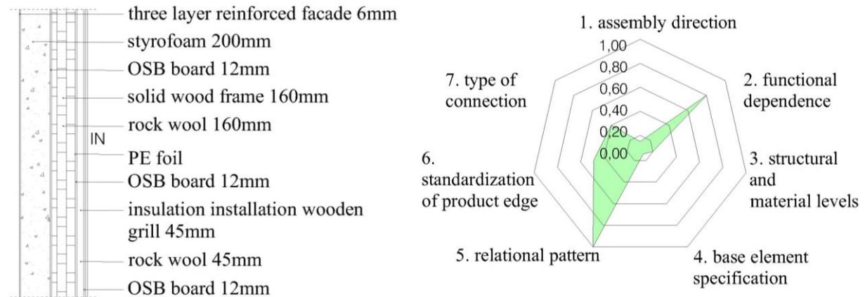
**Figure 3.** The section (left) and the overview of the main criteria of reversibility and the final score of the reuse potential of the 11 layers wall - existing façade system in wood (right) using method Durmisevic
