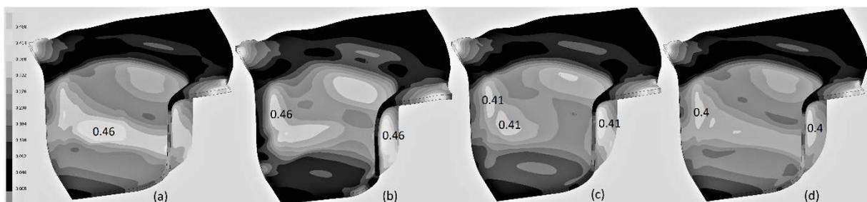
**Figure 7.** Process variations that give different forming limit distributions (a) Only pressure used (b) Only punch used (c) First half by pressure and last half by punch (d) only the lower corners by punch
