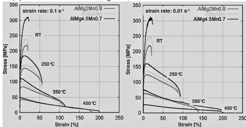
**Figure 2.** Stress-strain curves of some industrial Al-Mg-Mn alloys in tensile tests at various temperature and two level of strain rates [7].
