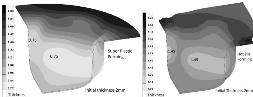
**Figure 6.** Thickness comparison of SPF (left) and HDF (right).
