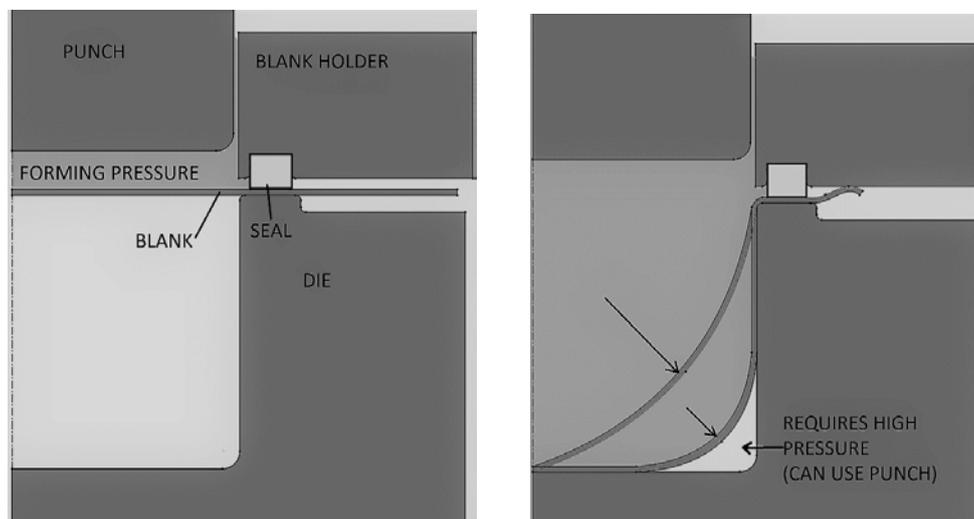
**Figure 1.** Schematic of hot die forming steps.
