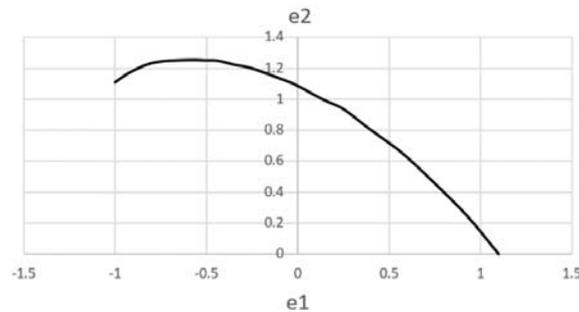
**Figure 4.** Forming limit diagram for Al EN-AW5083 at 500°C [5].
