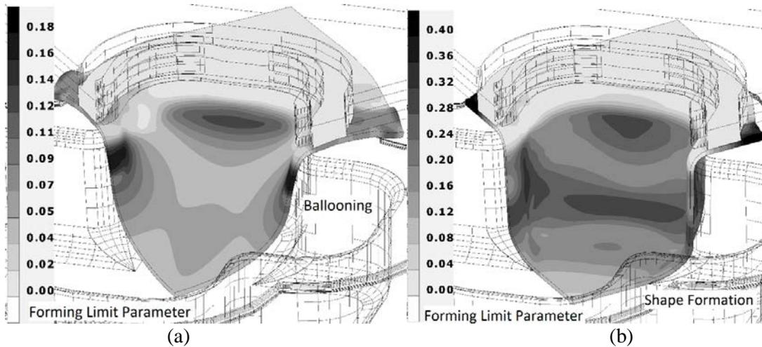
**Figure 5.** Process regime during HDF (a) Ballooning (b) Shape formation.
