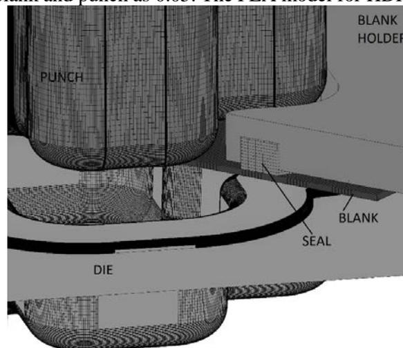
**Figure 3.** Finite element model for HDF.
