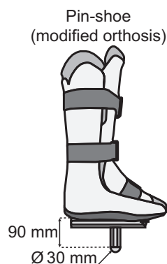
Fig. 1. Schematic drawing of one pin-shoe: an ankle-foot orthosis that blocks the ankle joint, modified to strongly reduce the support area of the foot. The vertical pin can be positioned along the foot.
