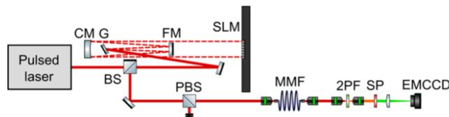
Fig. 1. Schematic of the experimental setup. The pulse shaper consists of (polarizing) beam splitters ((P)BS), a grating (G), a cylindrical mirror and folding mirror (CM/FM), and a spatial light modulator (SLM). The output facet of the multimode fiber (MMF) is imaged with a two-photon fluorescent screen (2PF), a short-pass filter (SP) and an electron-multiplying CCD camera (EMCCD).
