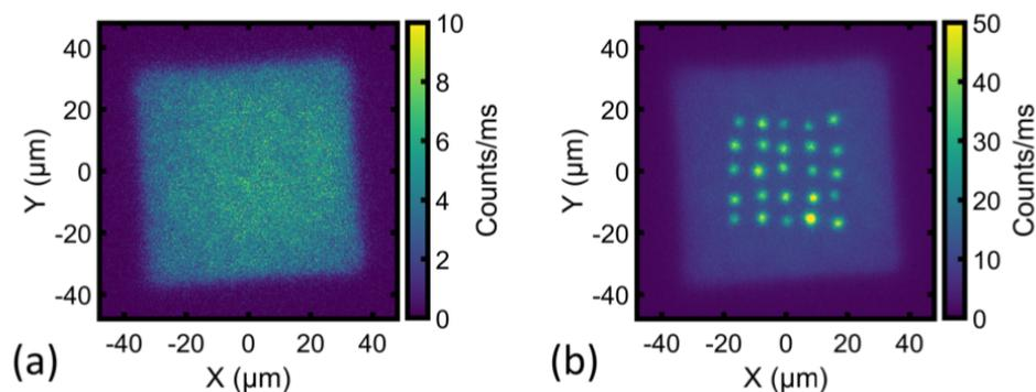
Fig. 2. (a) Nonlinear image of the output speckle pattern before optimizing the input pulse shape. (b) Composite nonlinear image of the output speckle pattern after selectively optimizing the input pulse shape for each of 25 speckles. This demonstrates grid scanning of an ultrashort pulse at the MMF output facet.
