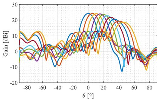
Fig. 2: Radiation pattern of the array antenna in azimuth plane for different scanning angles at 28 GHz.
