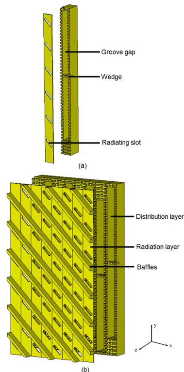
Fig. 1: Exploded view of (a) an element and (b) the array antenna.
