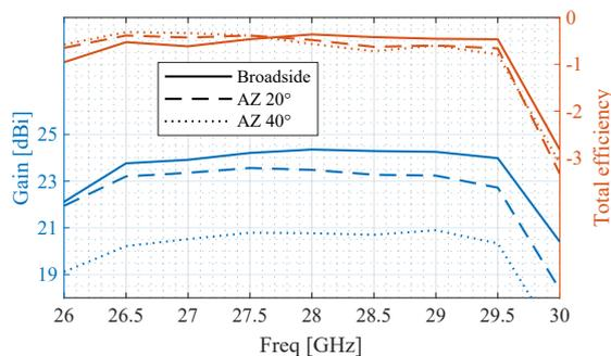
Fig. 3: Co-polar gain and total efficiency vs. frequency.
