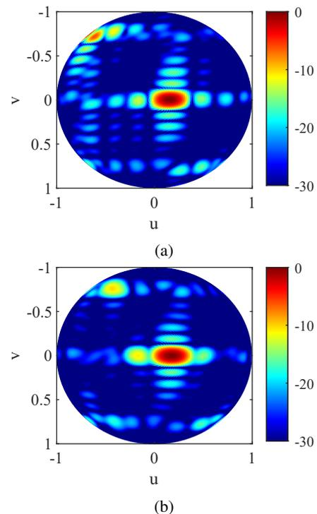
Fig. 4: UV-plane array radiation pattern when scanning to  $10^\circ$ , (a) without baffles, and (b) with baffles.
