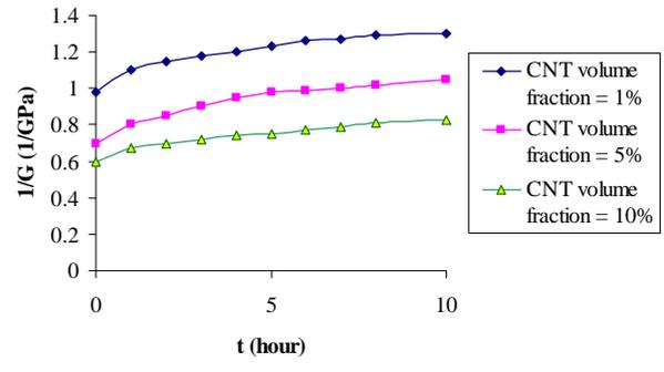
Fig. 3 variation of shear creep compliance with time for different values of volume fraction
