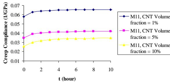
Fig. 6 variation of the axial creep compliance with time for different values of volume fraction
