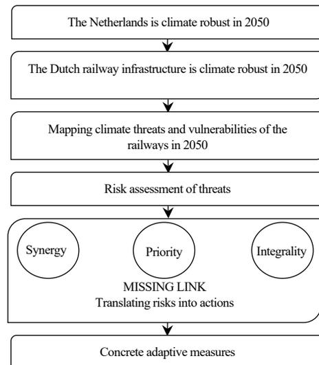
Figure 2: The CCA process at the Dutch railway infrastructure manager, including the identified ‘missing link’.
